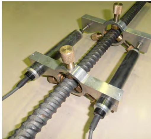
Photo 4: Jig used for a tensile test
