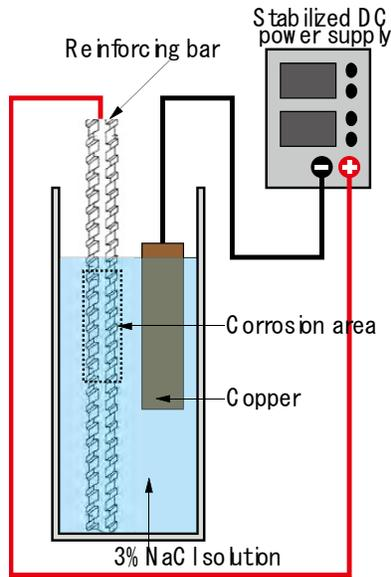
Figure 2: Outline of the corrosion accelerating test
