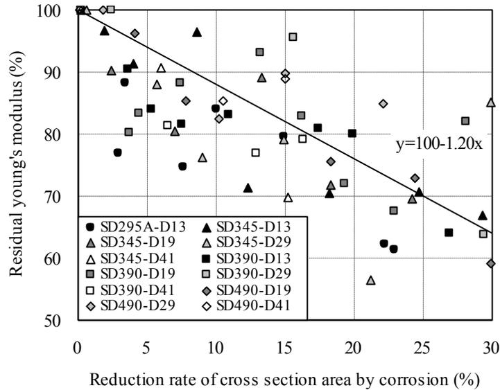
Figure 7. Relationship between the average corrosion loss ratio and the residual Young's modulus
