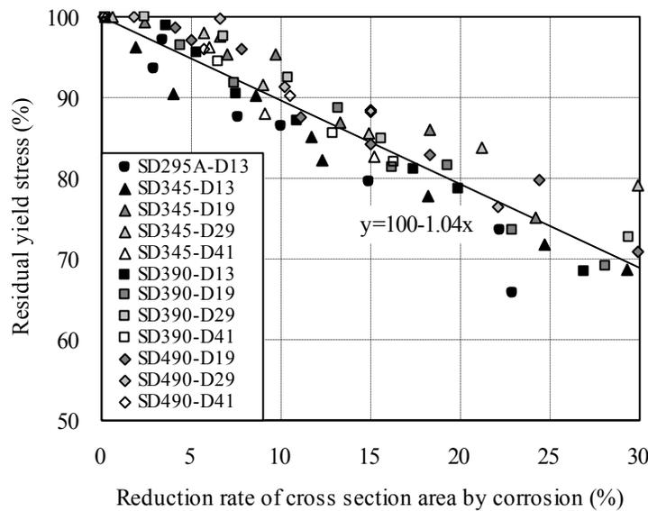
Figure 6. Relationship between the average corrosion loss ratio and the residual yield stress.
