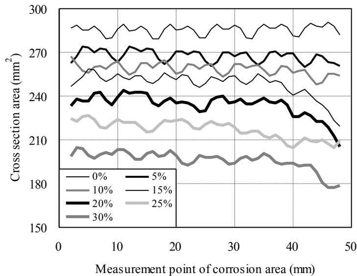
Figure 5: An example of the measurement about the cross section of a reinforcing bar (SD345-D19)
