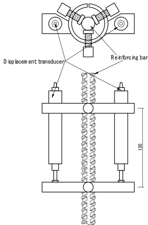
Figure 4: Detail of the jig used for a tensile test
