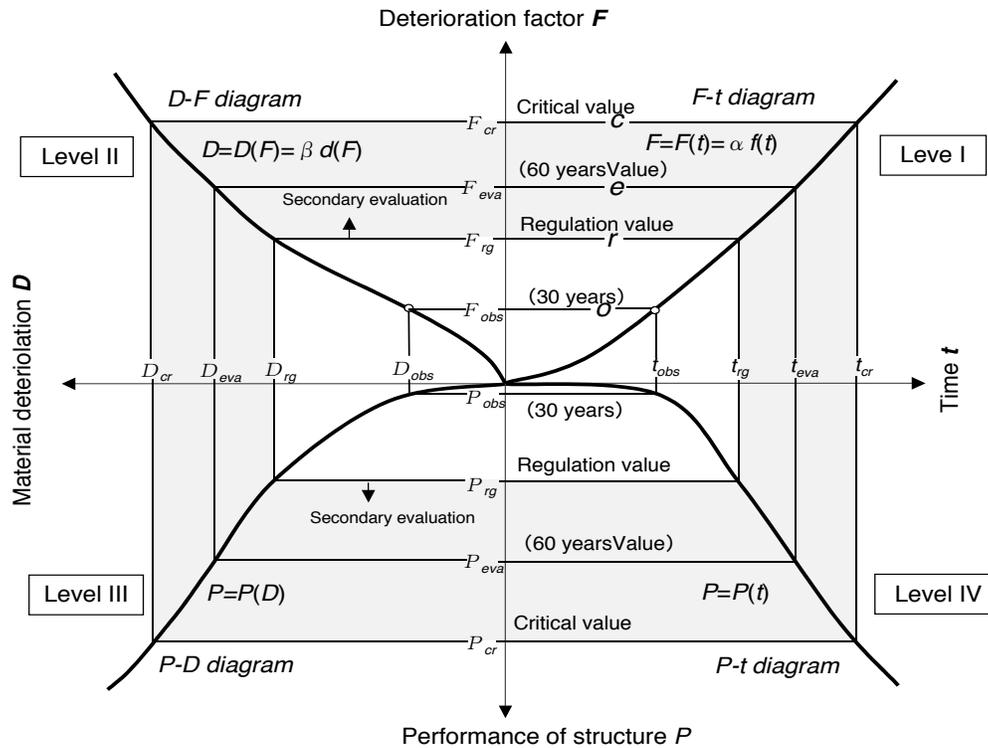
Figure 1: Integrity evaluation diagram of reinforced concrete structures ( $PDFt$  diagram)
