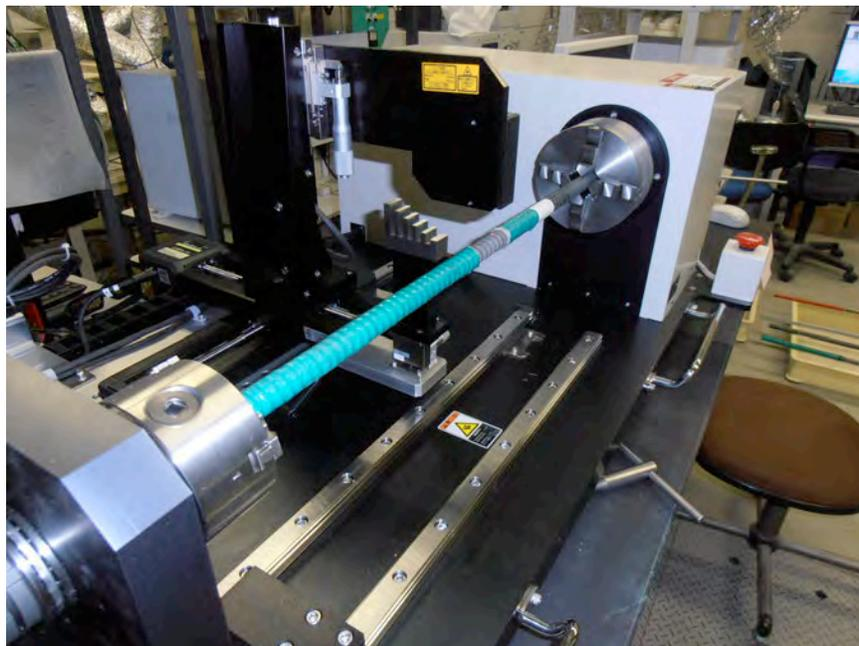
Photo 3: The equipment for measuring the cross-sections of a specimen
