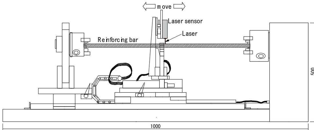
Figure 3: The equipment for measuring the cross-sections of a specimen (unit:mm)
