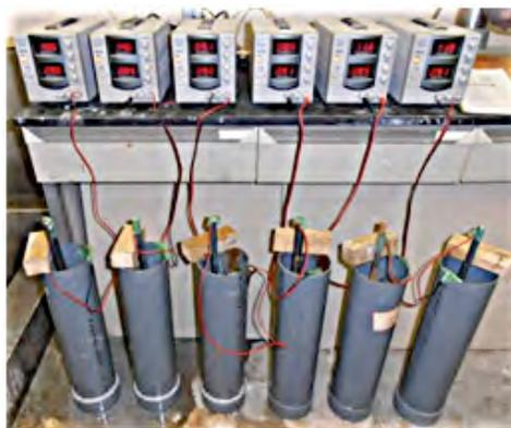
Photo 2: Corrosion accelerating test
