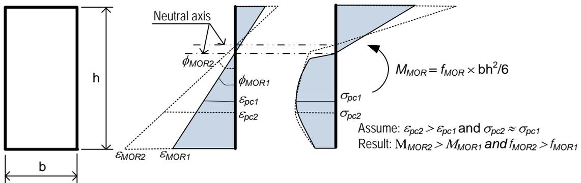
Fig. 5 – Influence of tensile strain capacity ( $\varepsilon_{pc}$ ) of UHPFRC on flexural strength ( $f_{MOR}$ )
