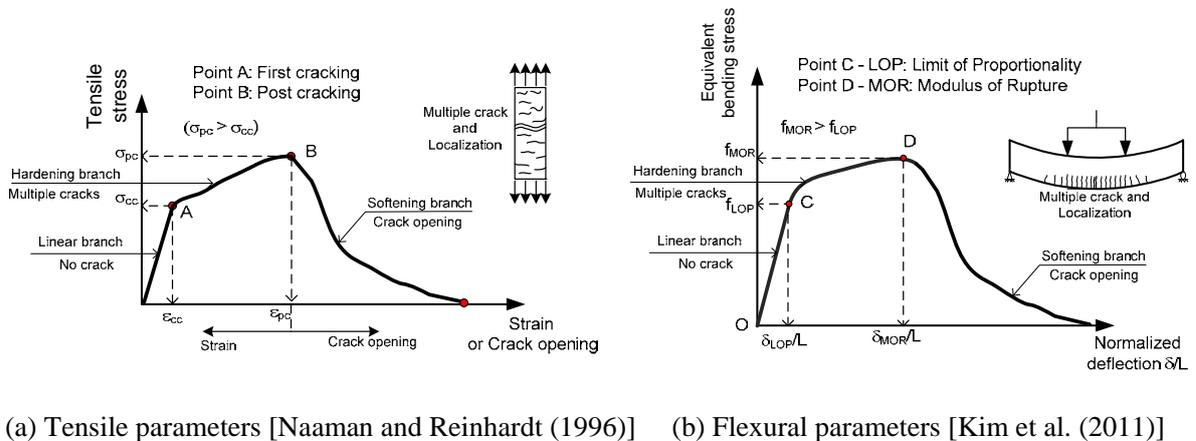
Fig. 3 – Mechanical parameters of UHPFRC
