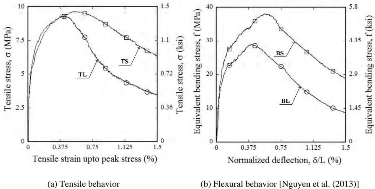
Fig. 4 – Effects of gauge length on the tensile and flexural behavior of UHPFRC
