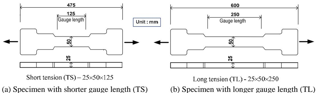
Fig. 1 – Geometry of tensile specimens
