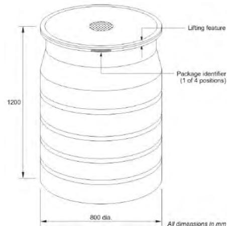
Figure 2. Schematic illustration of an ILW container (NDA, 2008).
