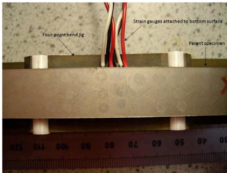
Figure 3. A parent specimen fitted on a four-point bend jig.
