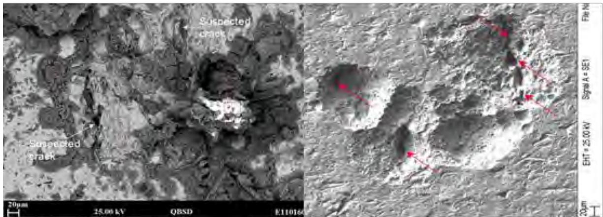
Figure 4. Morphology of specific pits and cracks before clean-up (Left image) and after clean-up (Right image) with arrows indicating cracks.
