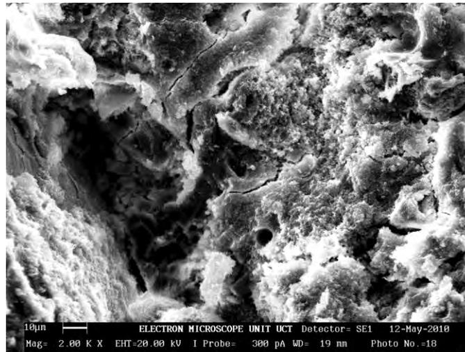
Figure 4: Unsealed concrete after exposure to 450°C
