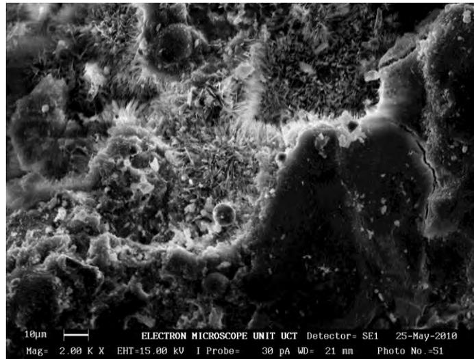
Figure 2: Evidence of CSH formation after exposure to 225°C for 7 days in a sealed environment
