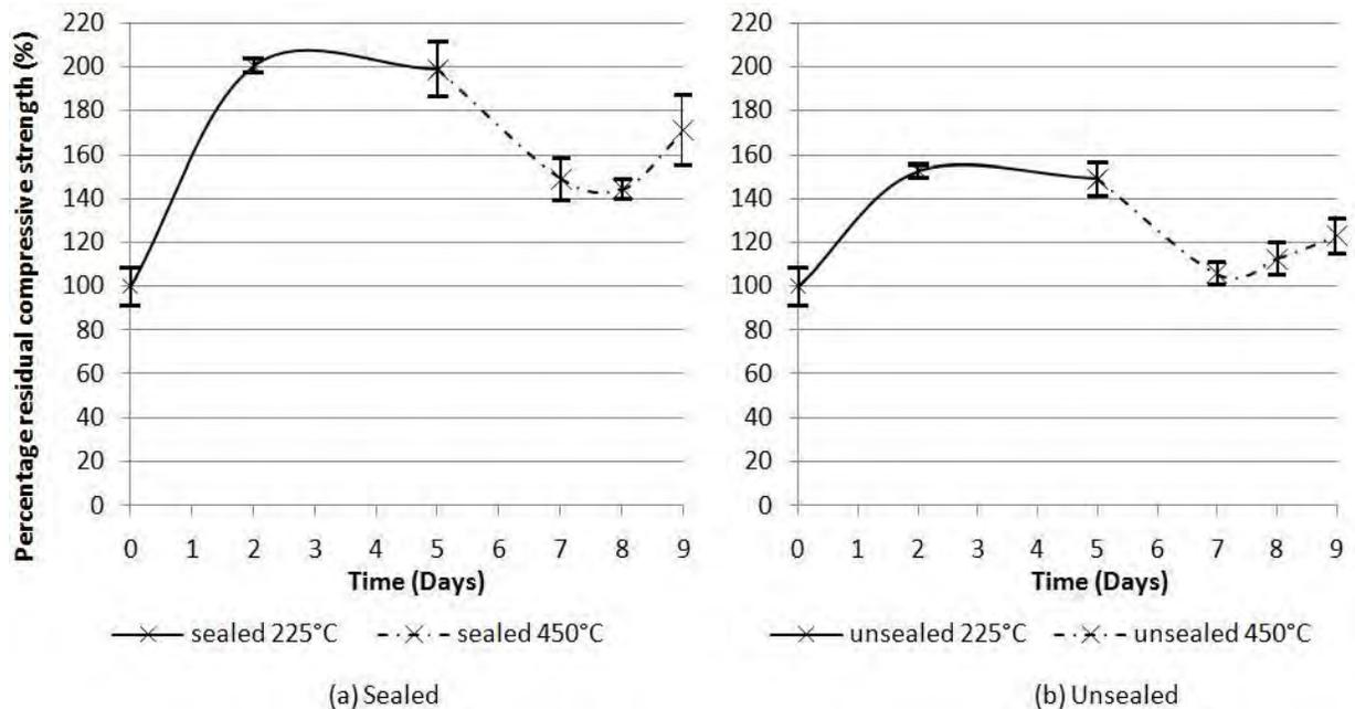
Figure 1: Residual Compressive Strengths of Concrete After Thermal Exposure (a) Sealed and (b) Unsealed, McCormick (2011)
