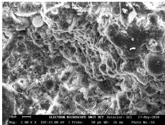
Figure 3: Sealed concrete after 225°C exposure for 7 days
