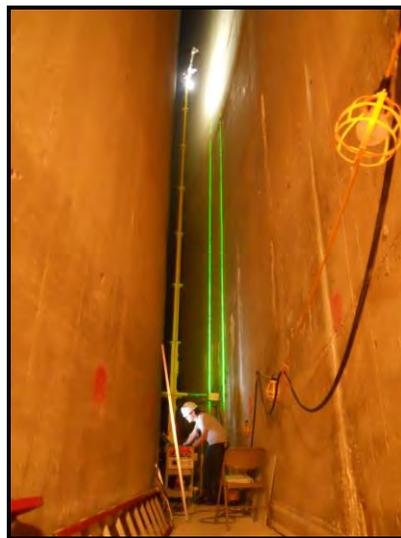
Figure 2. Digital Image System with Camera Mast Stand and Linear Lasers
