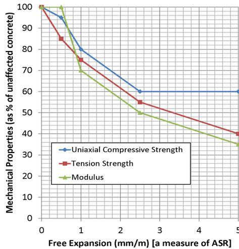
Figure 1. Residual mechanical properties vs. free expansion, from ISE (1992), Table 4.
