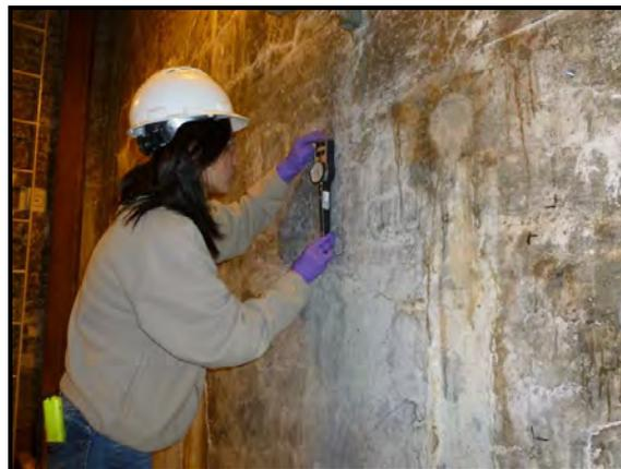
Figure 8. Measurements with Mechanical Strain Gage
