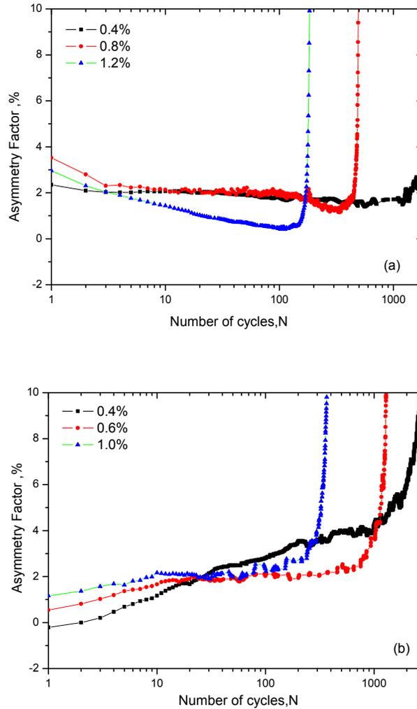
Fig.3 Variation of the asymmetry factor with the number of cycles at (a)773K and (b)873K
