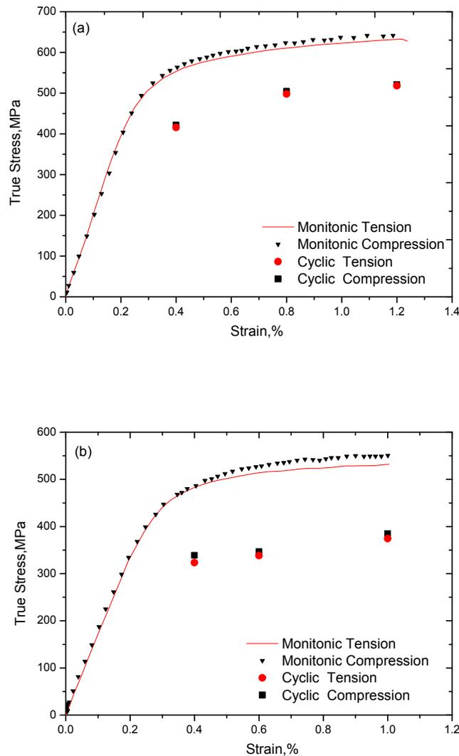
Fig.4 The monotonic as well as cyclic stress-strain relationship at (a)773K and (b)873K
