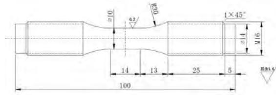
Fig. 1 Low cycle fatigue specimen
