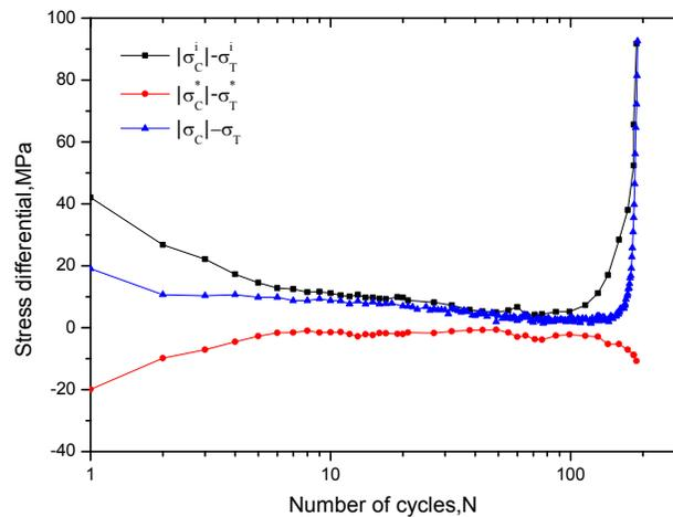
Fig.6 Evolution of strength differential of back stress, effective stress and peak stress during cycling
