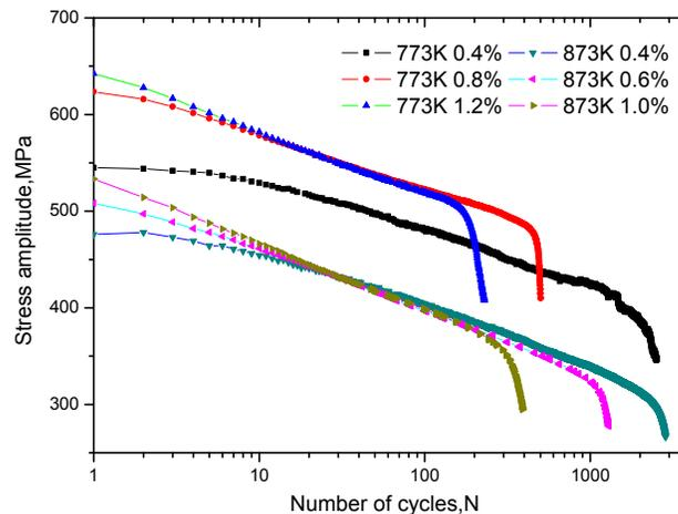
Fig.2 Evolution of the stress amplitude during LCF testing of X12 at 773K and 873K
