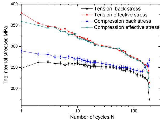
Fig.5 Evolution of back and effective stress during cycling in LCF tested ( T=773K and  $\Delta\varepsilon_t = 1.2\%$  )
