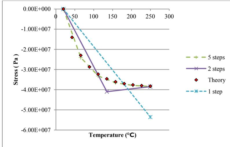
Figure 3: Evolution of stress on a restrained element
