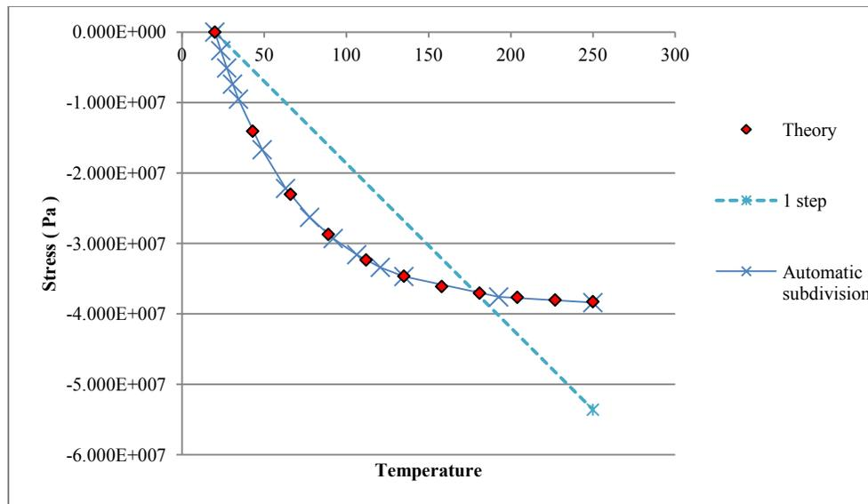
Figure 4: Evolution of stress with automatic subdivision of time steps
