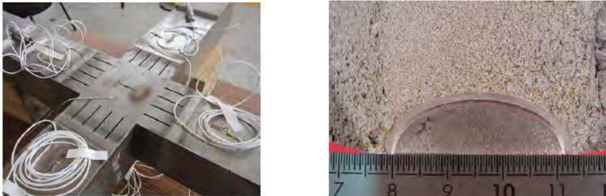
Figure 3. CEA WPS cruciform specimen (with a view of typical flaw after fracture).
