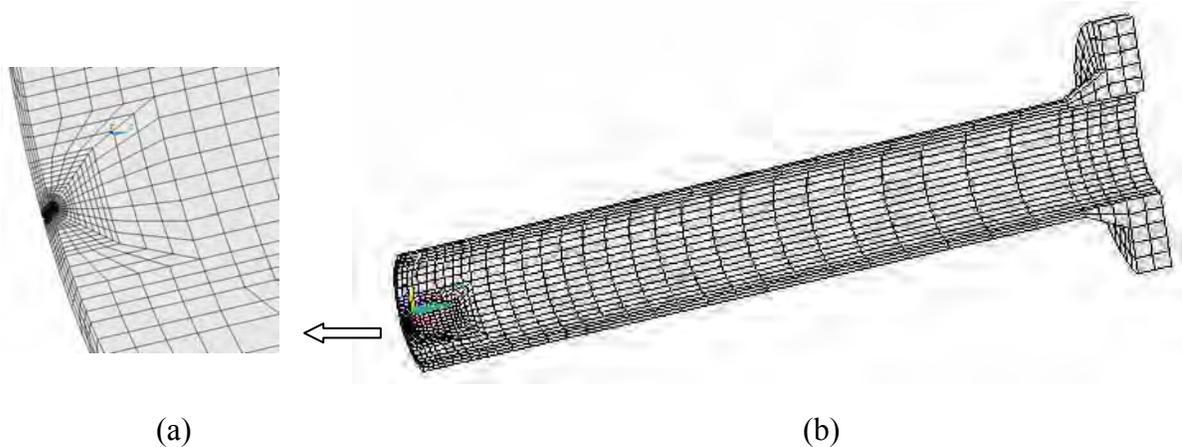
Fig.2: (a) Zoomed view of crack region and (b) one-quarter finite element model of pipe-flange assembly.
