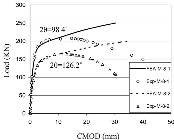
Fig.4: Comparison of load-CMOD response obtained from FE analysis with experimental data.
