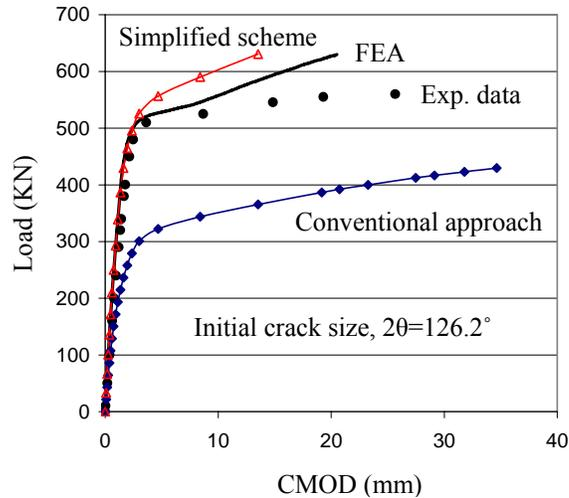
Fig.6: Comparison of load-CMOD response, of a piping system having finite compliance, obtained from FE analysis with experimental data.
