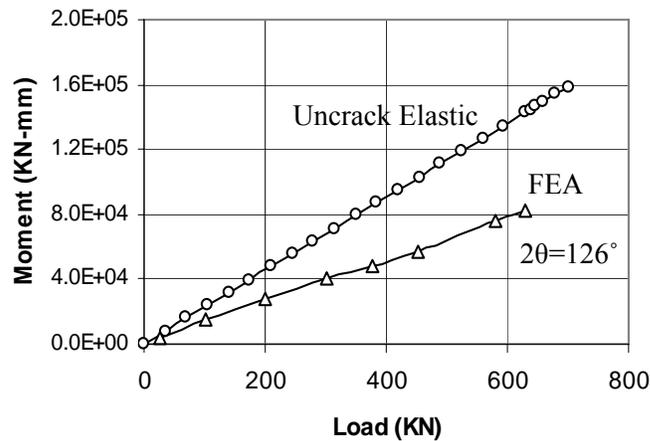
Fig.5: Comparison of bending moment obtained from uncracked elastic analysis (conventional approach) with the actual moment obtained from detailed elastic-plastic FE analysis.
