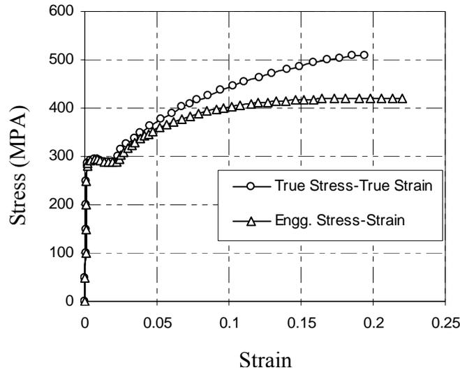
Fig.3: Stress-strain data of SA-333 Gr-6 material (Chattopadhyay et al., 2000).
