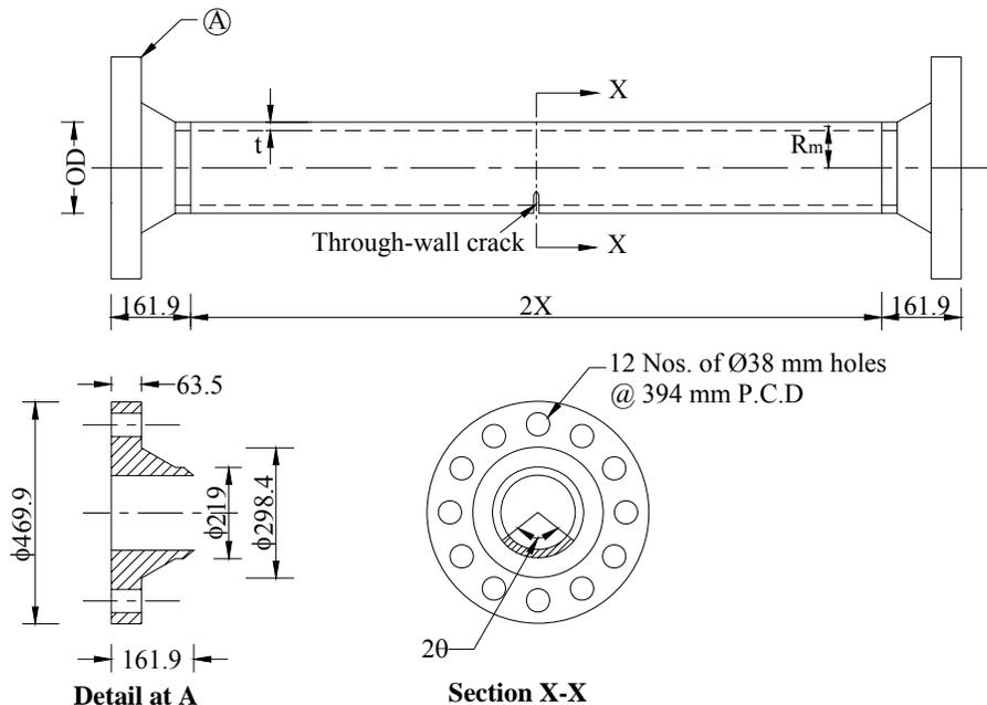
Fig.1: Details of pipe assembly with pipe having a through-wall crack at the centre. All dimensions are in mm.
