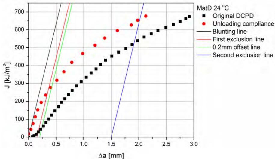
Figure 2. Comparison of J-R curves of original DCPD result and EUC for MatD at 24 °C.
