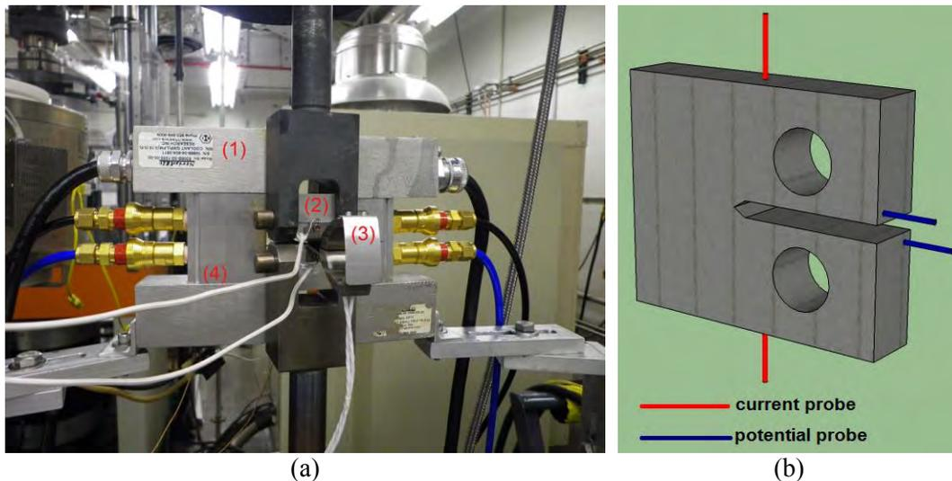
Figure 1. (a) Fracture toughness testing setup: (1) infrared heating, (2) C(T) specimen, (3) displacement gage, (4) potential probes; (b) location of current and potential probes for DCPD acquisition.
