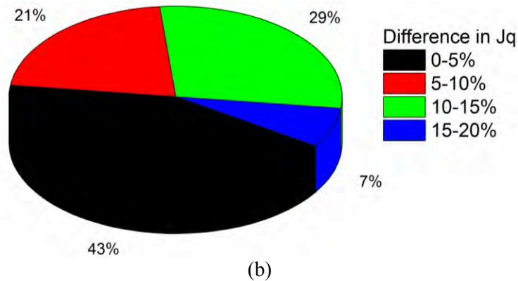
Figure 4. (a) Comparison of post-adjustment DCPD  $J_q$  with EUC or normalization  $J_q$ ; (b) statistical analysis of the difference in  $J_q$  between post-adjustment DCPD results and EUC or normalization results.
