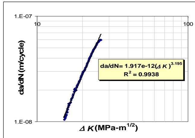
Figure 2. Evaluation of Paris constants (C and m) from  $da/dN$  versus  $\Delta K$  curves for SS304LN
