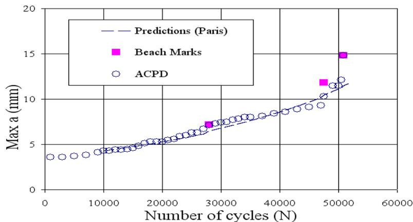
Figure 6. Comparison for tested FCG behavior with predictions for SSPB 6-9
