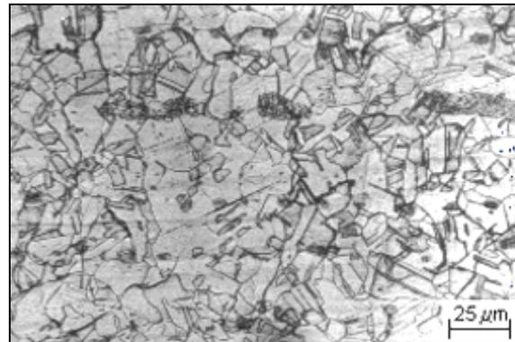
Figure 1. Typical microstructure of the investigated SS 304 LN material
