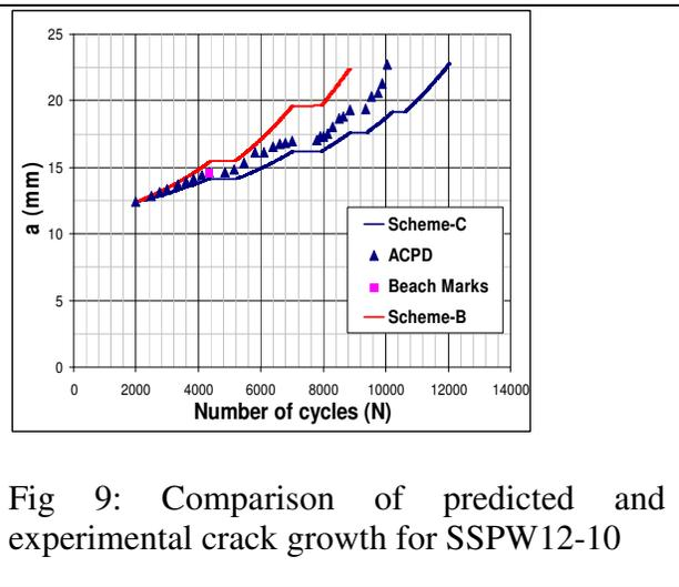
Fig 9: Comparison of predicted and experimental crack growth for SSPW12-10
