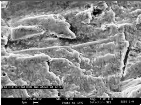
Fig 7a: Fatigue surface near notch (SSPB6-9)
