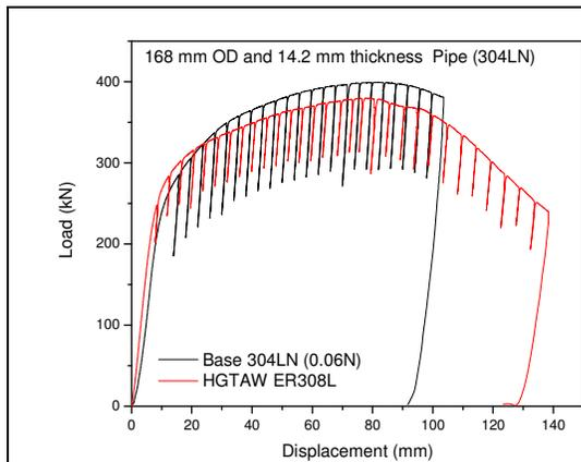
Fig 10: Load verses load line displacement of base and weld (hotwire GTAW)
