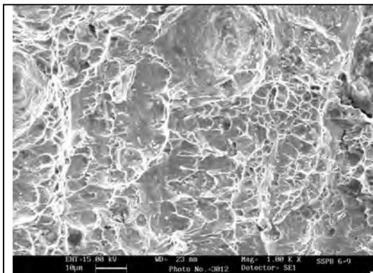
Fig 12: Fracture surface of the base metal (pipe)
