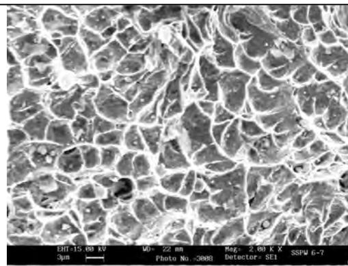
Fig 13: Fracture surface of the weld metal (GTAW)
