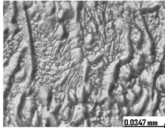
Fig 1d: Weld of cold wire GTAW (Conventional V-Groove)
