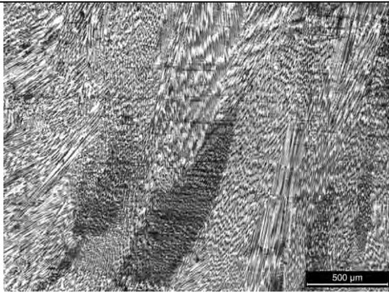
Fig 1e: Weld of Hot wire GTAW (Narrow Gap)
