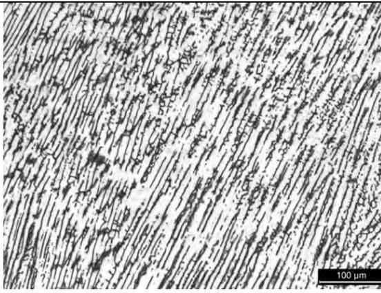
Fig 1f: Dendritic structure in weld of Hot wire GTAW (Narrow Gap)-higher magnification
