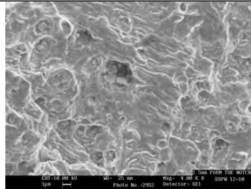
Fig: 7f: Fatigue fracture surface (SMAW)-SSPW12-10
