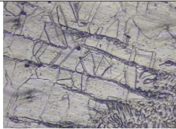
Fig 1b: Heat Affected Zone of cold wire GTAW (Conventional V-Groove)
