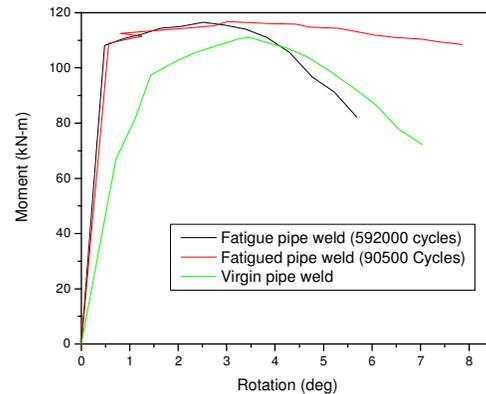
Fig 11: Load verses load line displacement of virgin and fatigue tested pipe weld with crack
