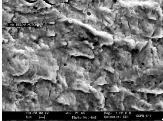
Fig: 7c: Fatigue surface near notch (cold wire GTAW)-SSPW6-7
