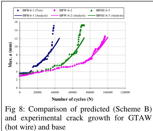
Fig 8: Comparison of predicted (Scheme B) and experimental crack growth for GTAW (hot wire) and base
