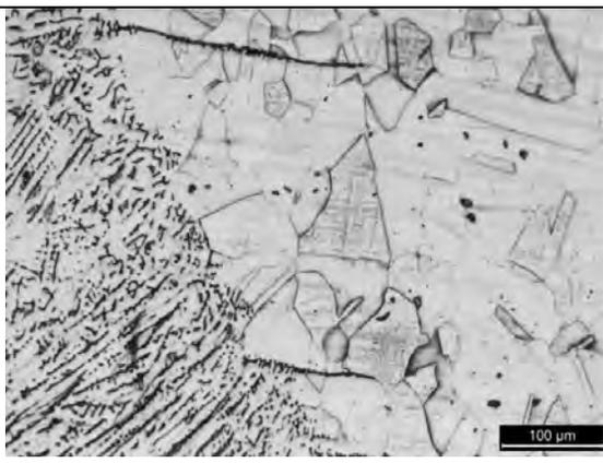
Fig 1h: Weld and Heat Affected Zone of hot wire GTAW (Narrow Gap)-higher magnification
