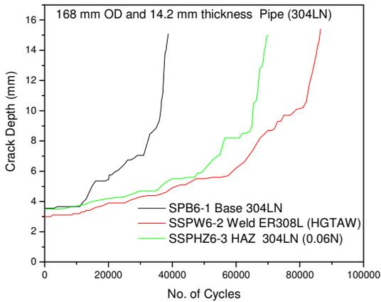
Fig 3: Crack growth in narrow gap welds produced by hot wire GTAW
