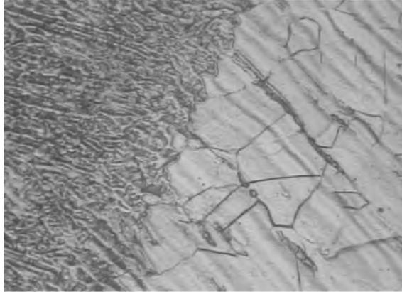
Fig 1c: Weld and Heat Affected Zone of cold wire GTAW (Conventional V-Groove)
