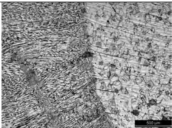
Fig 1g: Weld and Heat Affected Zone of hot wire GTAW (Narrow Gap)
