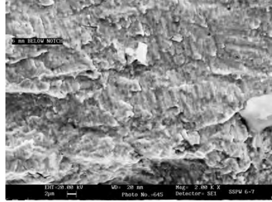
Fig: 7d: Fatigue surface away from notch (cold wire GTAW)-SSPW6-7
