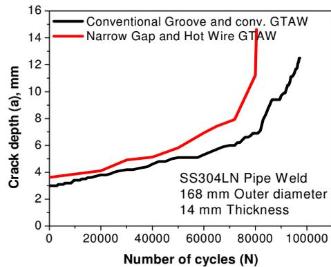
Fig 6: Comparison of crack growth cold wire (V-groove) and hot wire (narrow gap) GTAW
