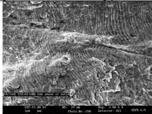
Fig 7b: Fatigue surface away from notch (SSPB6-9)
