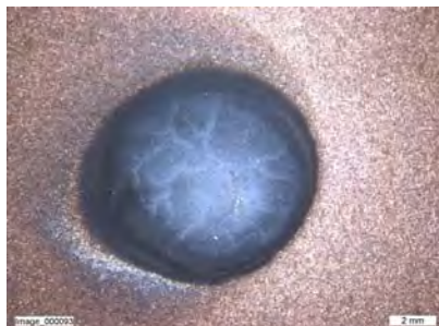
Fig. 11d: Crack network inside the hot spot after 525 \cdot 10^3 CTS.
