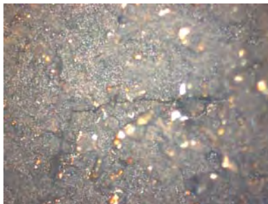
Fig. 11b: Crack network after 223 \cdot 10^3 CTS top side surface.
