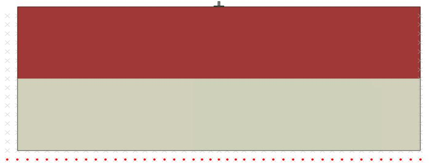
Figure 6: ABAQUS model of spent fuel cask on concrete storage pad resting on a two layer soil column. The three component acceleration time series are applied to the red nodes shown.
