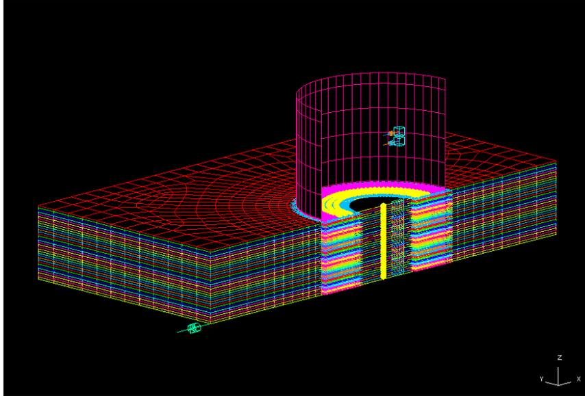
Figure 3: Liquid Natural Gas Tank SSI Simulation Finite Element Model including Fluid and Tank Wall Uplift, Willford et al, (2010)
