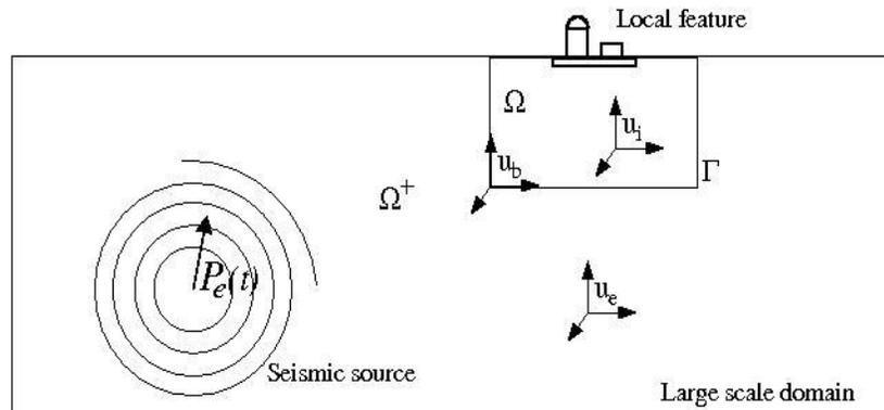
Figure 5: Geometry of the soil-foundation-structure system (Jeremic et al. 2012).
