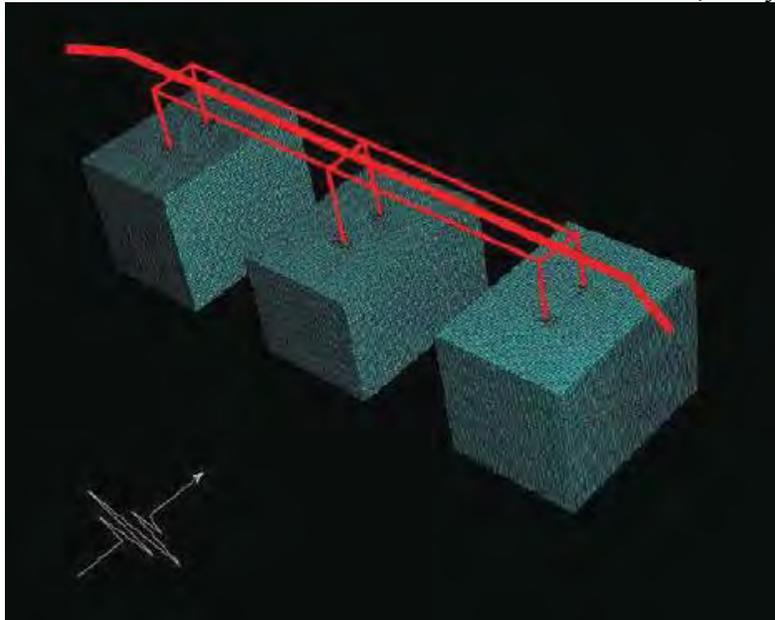
Figure 2: Detailed Three Bent Prototype Soil-Structure-Foundation Interaction Finite Element Model, Jeremic et al. (2009)
