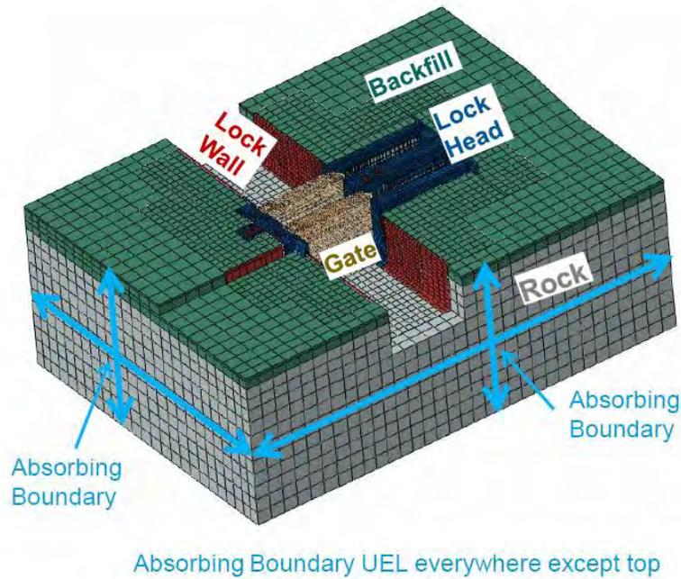
Figure 1: Finite Element Model of Panama Canal 3<sup>rd</sup> set of Locks, Barry (2012)
