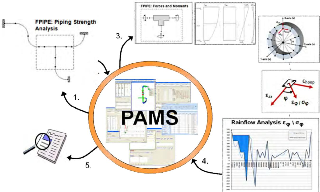
Figure 1. Work flow for the fatigue analysis
