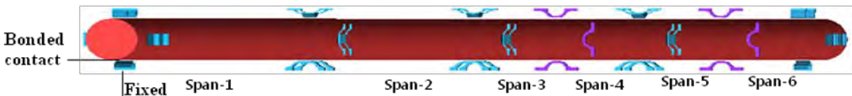
Figure 4. Fuel rod supported by 1x1 spacer grids
