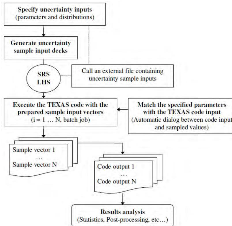
Figure 1. Operation of a TEXAS-SAUNA coupled system.
