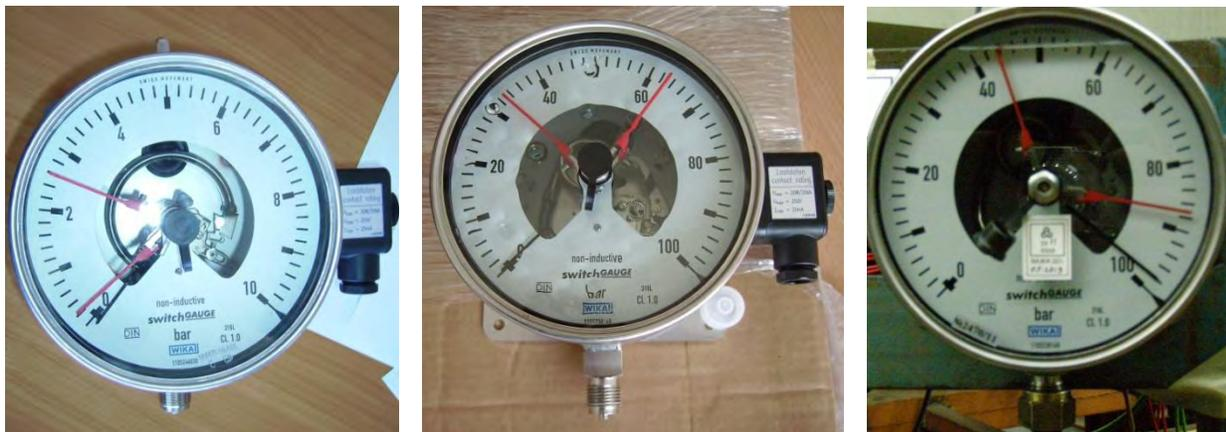
Figure 1 View of two samples of pressure gauges with magnetic snap-action contacts
