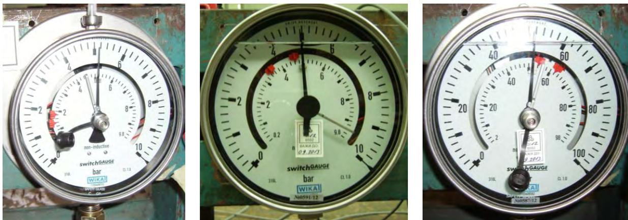
Figure 2 View of two samples of pressure gauges with reed switch contacts
