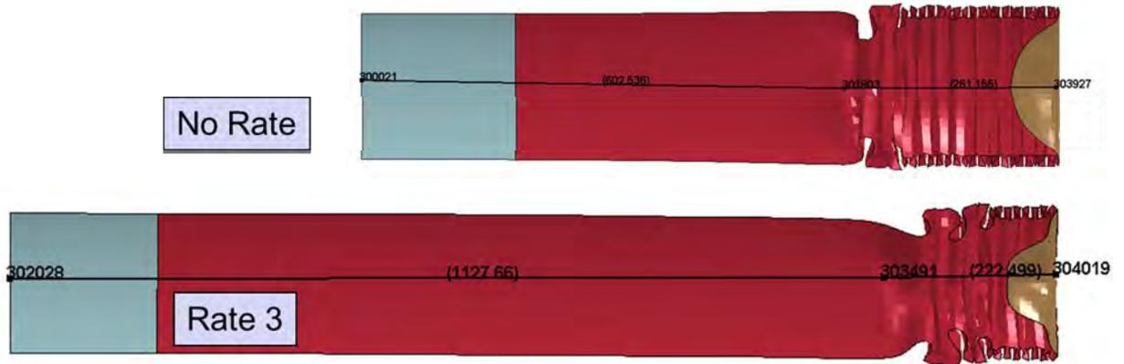
Figure 4 Comparison of stainless steel projectile final deformation without (top) and with (bottom) Cowper-Symonds strain rate model.
