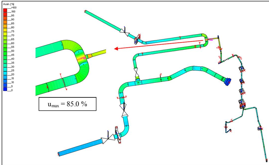
Figure 4. Stress utilization factors for analysis A1: RSMA with enveloped raw spectra
