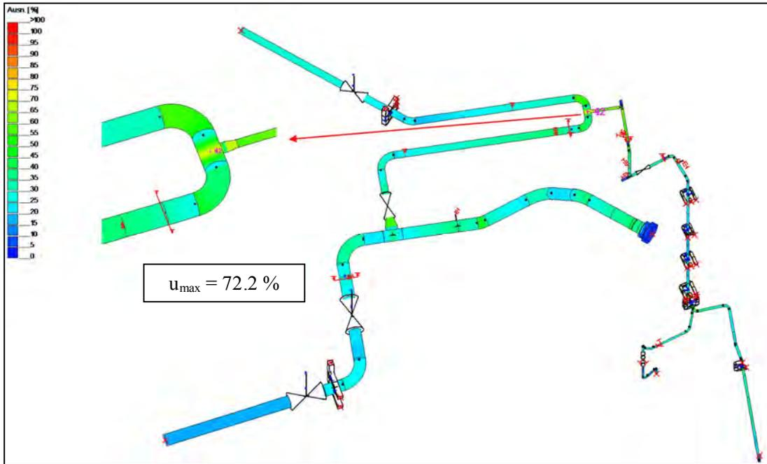
Figure 6. Stress utilization factors for analysis A3: RSMA with multi-support excitation with raw spectra
