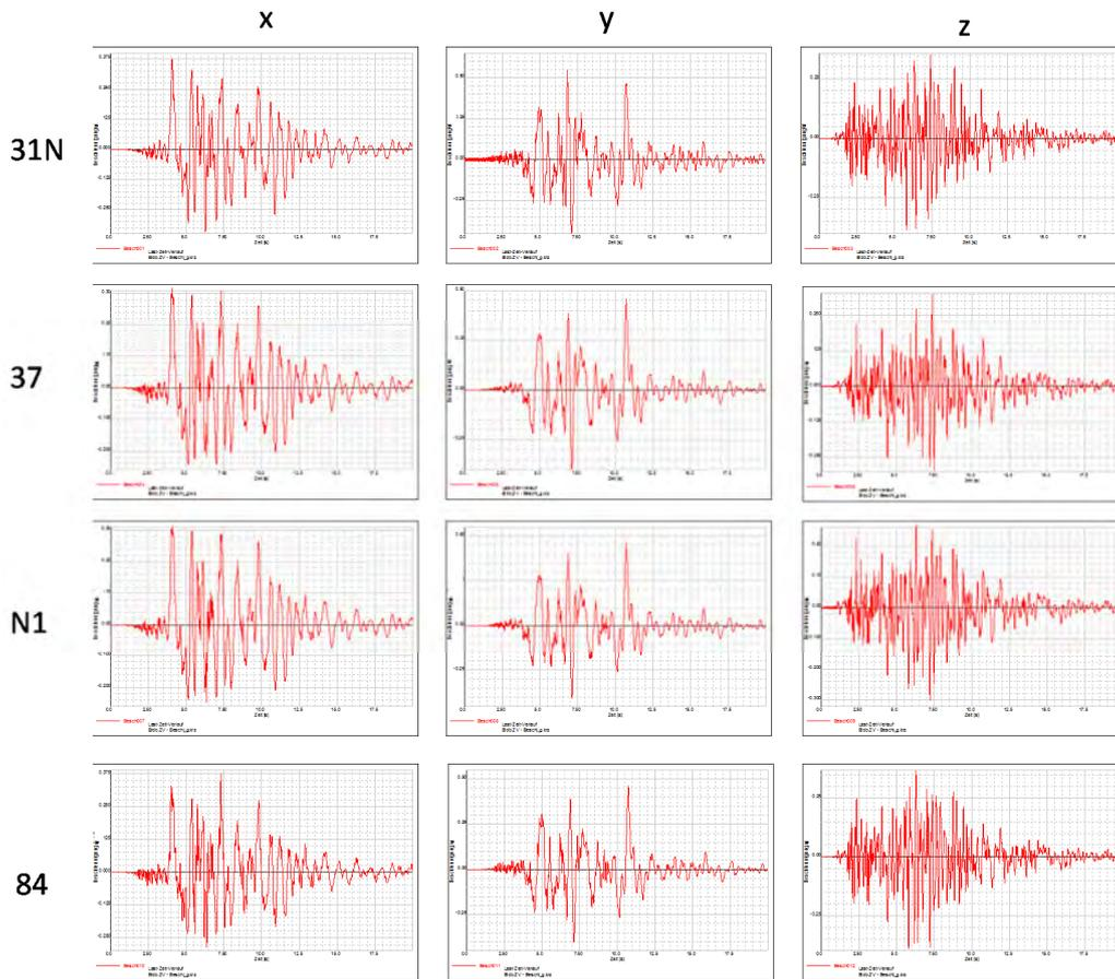
Figure 2. Acceleration time histories at four locations derived from reactor building analysis
