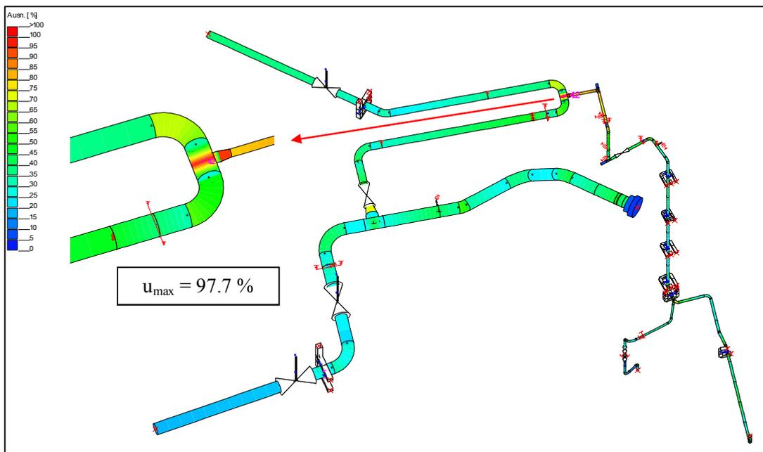
Figure 5. Stress utilization factors for analysis A2: RSMA with enveloped and smoothed spectra
