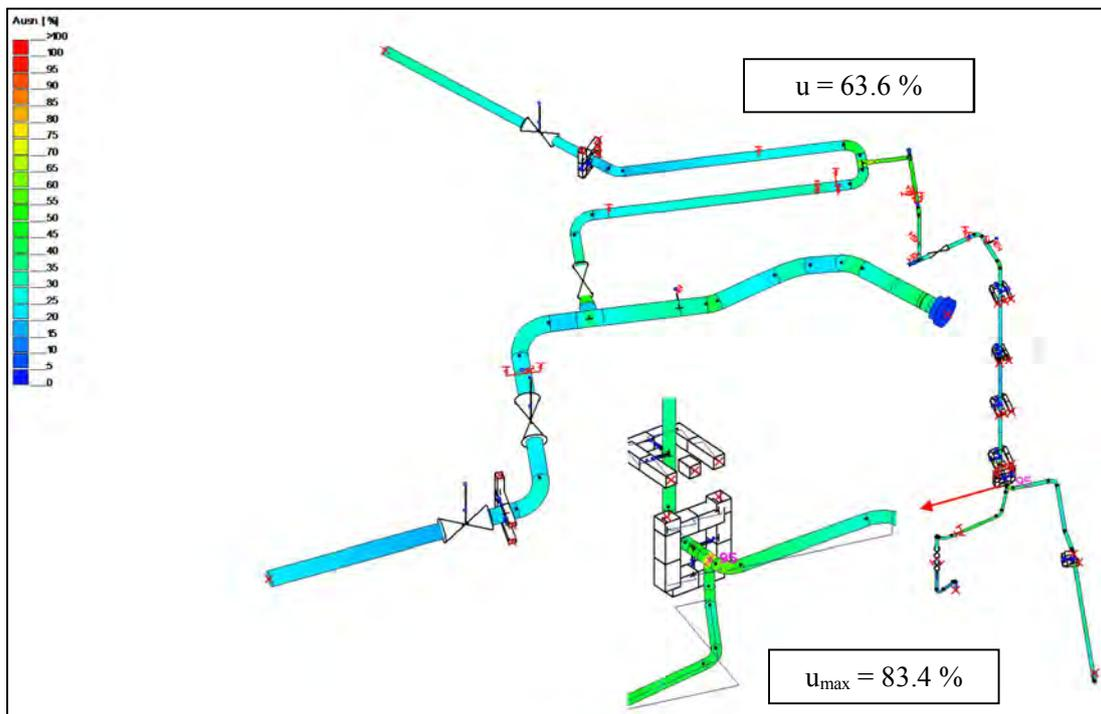
Figure 7. Stress utilization factors for analysis A4: Time-history analysis with multi-support excitation
