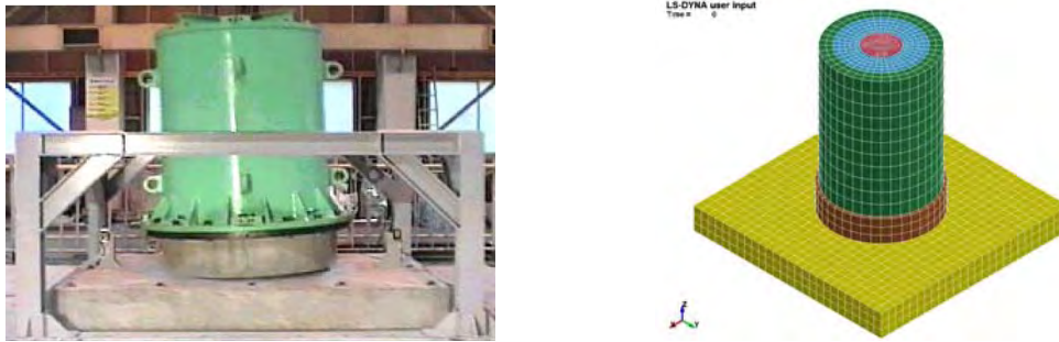
Fig. 2 (a) 1/3 Scale model cask for shaking table test (Shirai et al., 2003) and (b) its FE model.
