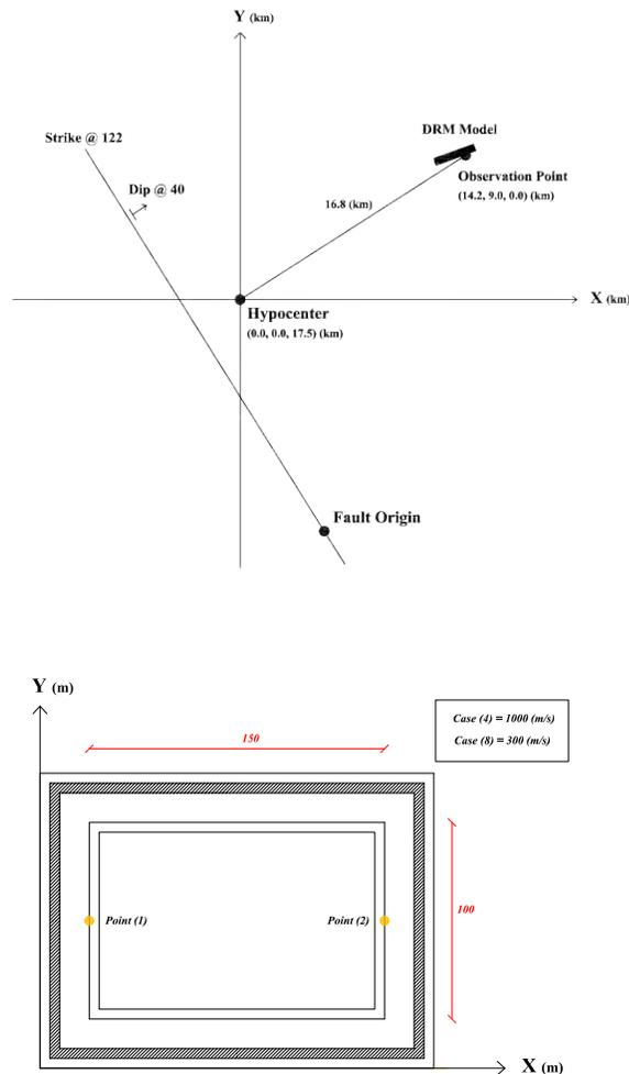
Figure 1: Upper: Analytic model (Green's functions) setup, with locations of hypocenter, epicenter and the DRM model; Lower: Location of observation points 1 and 2, at the edge of foundation model.
