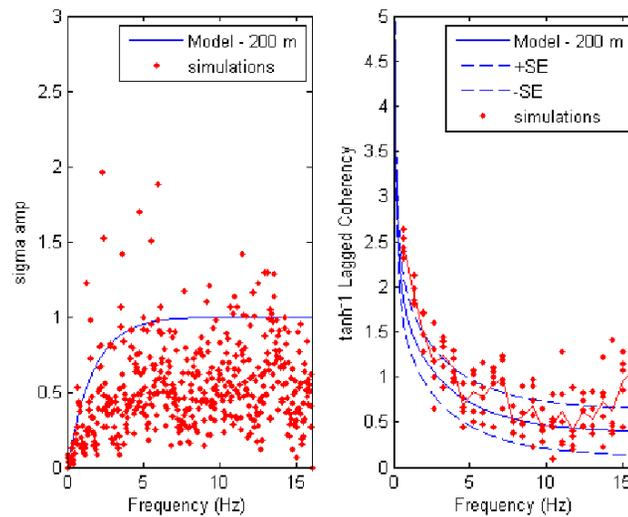
Figure 4: Validation of case 5 (soil) using location 1 as a seed against the selected  $\sigma_{\Delta A}$  (left) and  $\gamma_{pw}$  (right) models. Solid blue lines are the selected  $\sigma_{\Delta A}$  and  $\gamma_{pw}$  models, while dashed lines on the right are model  $\pm\sigma$ . Red dots are the estimate of the metric comparing the seed to the 5 simulations. The solid red line on the right is a running mean of the estimated plane wave coherency.
