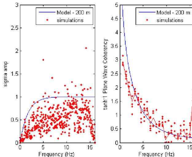
Figure 3: Validation of case 1 (rock) using location 1 as a seed against the selected  $\sigma_{\Delta A}$  (left) and  $\gamma_{pw}$  (right) models. Solid blue lines are the selected  $\sigma_{\Delta A}$  and  $\gamma_{pw}$  models. Red dots are the estimate of the metric comparing the seed to the 5 simulations. The solid red line on the right is a running mean of the estimated plane wave coherency.
