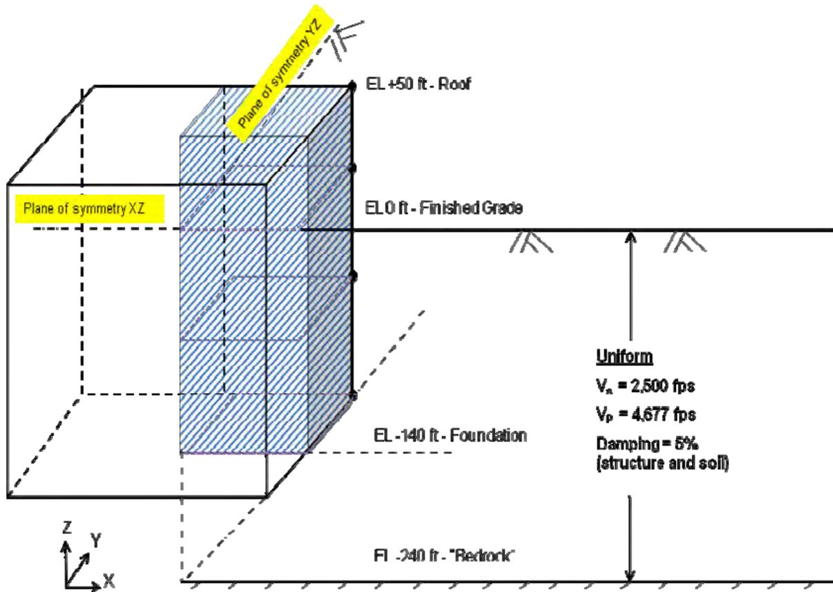
Figure 3. 3D view of the Deeply Embedded Structure with Two Planes of Symmetry used for Modeling.
