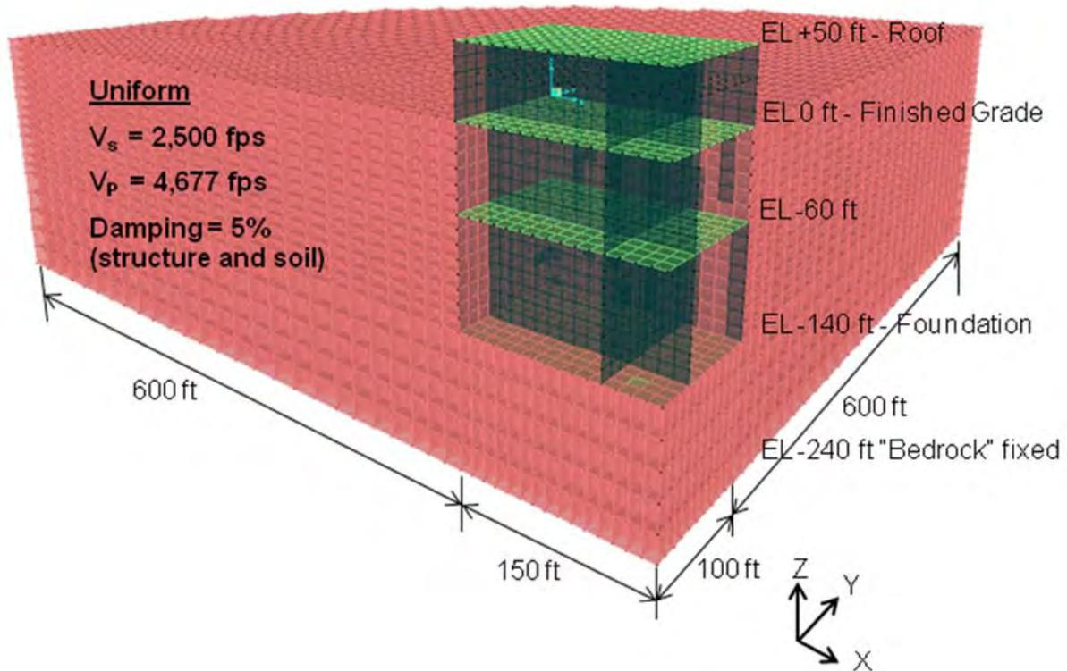
Figure 4. SAP2000 Soil and Structural Model Geometry and Properties.
