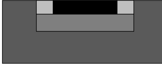
Figure 1. Scheme of the sample model: rigid basement embedded into two-layered soil pillow in rocky half-space
