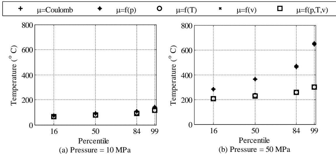
Figure 8: 16<sup>th</sup>, 50<sup>th</sup>, 84<sup>th</sup> and 99<sup>th</sup> percentile values of the maximum temperature on the sliding surface of the FP bearing with different levels of static axial pressure subjected to 30 ground motions
