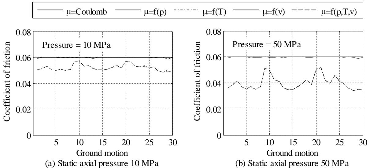
Figure 5: Averaged values of the coefficient of friction over the duration of strong shaking
