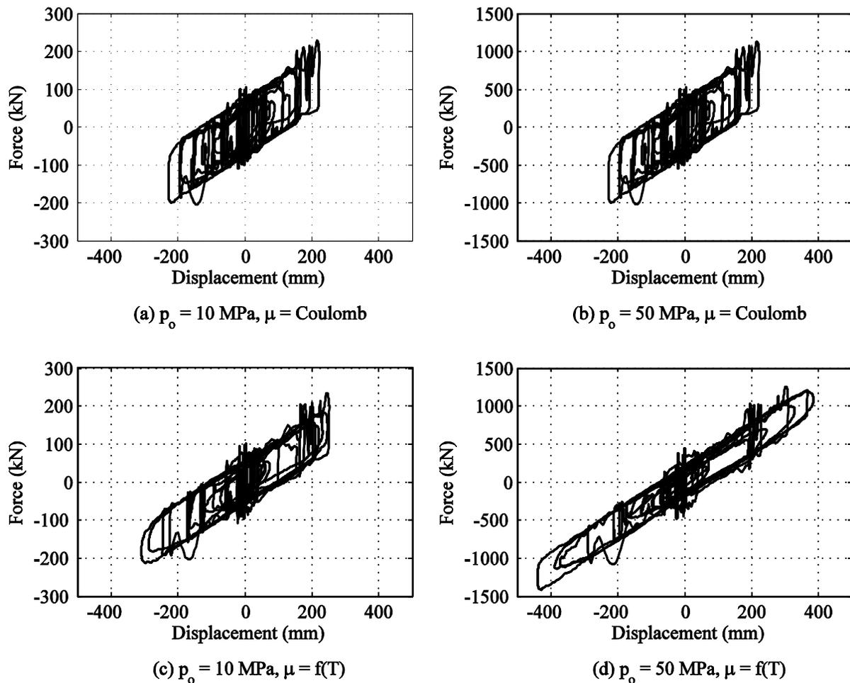
Figure 6: Force-displacement response of an FP bearing with different levels of static axial pressure and friction models
