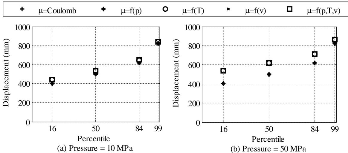
Figure 7: 16<sup>th</sup>, 50<sup>th</sup>, 84<sup>th</sup> and 99<sup>th</sup> percentile values of displacement demand on the FP bearing with different levels of static axial pressure subjected to 30 ground motions
