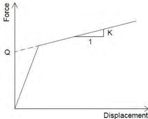
Figure 2: Lateral force-displacement relation of an FP bearing
