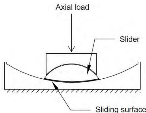
Figure 1: A section through a Friction Pendulum™ (FP) bearing
