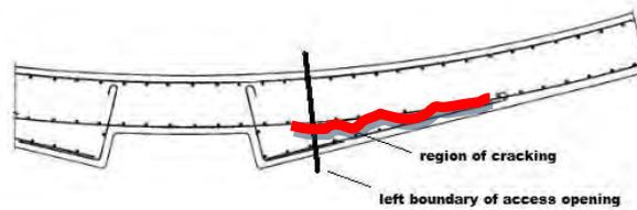
Figure 1. Cracking in Flute shoulder Region to the Left of the Construction Opening
