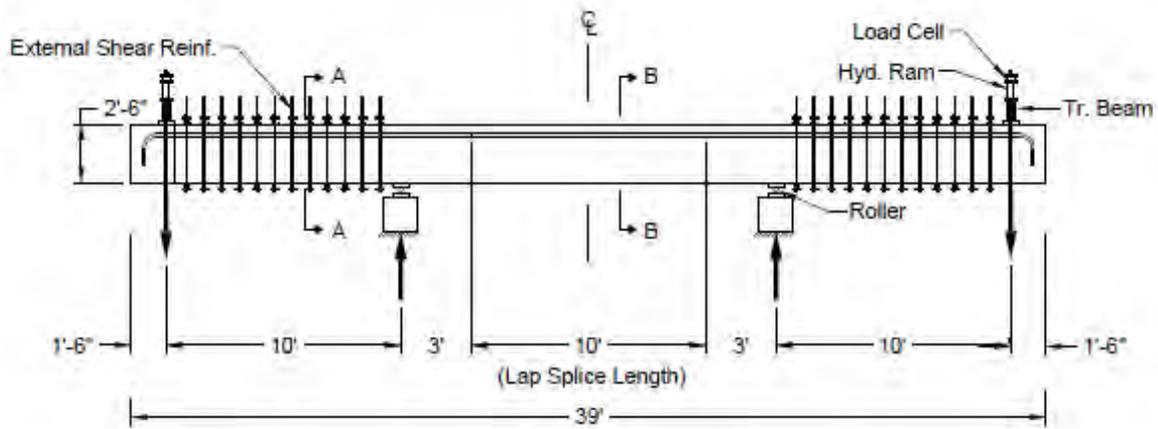
Figure 3 Test Girder, Series A Purdue Tests (120 in splice)
