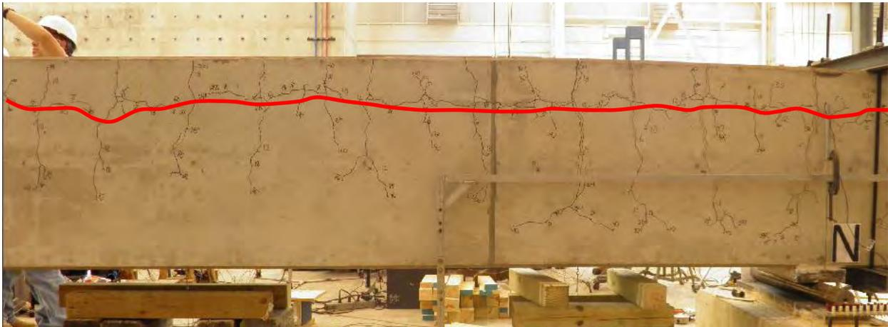
Figure 4 Typical Pattern of Flexural Cracks and Bursting Cracks Highlighted Resulting in Laminar Cracking (Purdue Testing)
