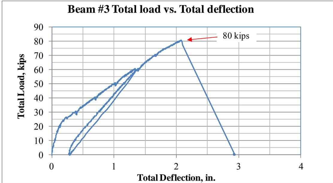
Figure 7 Total Load vs. Total Deflection for Beam 3 (with a cold joint) at University of Kansas
