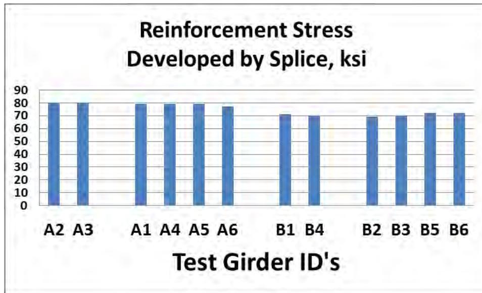
Figure 6 Maximum Unit Stress Reached by Lap Splices at Purdue
