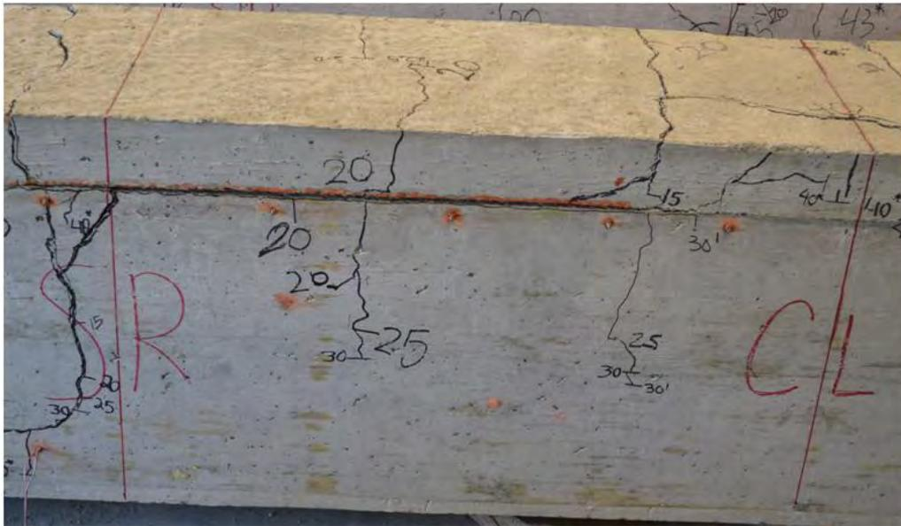
Figure 8 Beam 3 Failure with Wide Horizontal Cracks Along Cold Joint, University of Kansas
