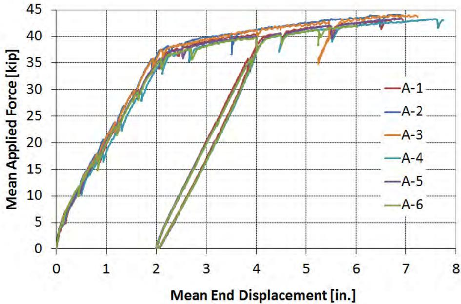
Figure 5 Force-Displacement for A-Series (120 in Laps) of Tests at Purdue
