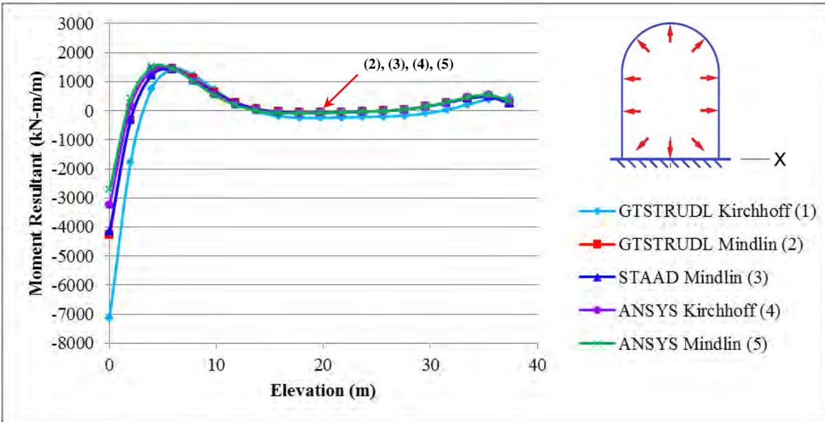
Figure 5. Moment Resultant about X at Various Containment Elevations
