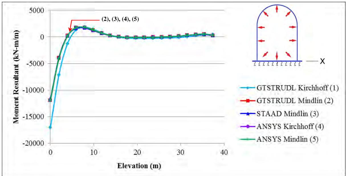
Figure 7. Moment About X Axis at Various Containment Elevations
