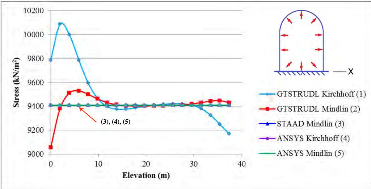
Figure 6. Middle Surface Vertical Stress at Various Containment Elevations
