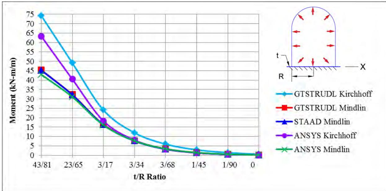
Figure 9. Fixed End Moment About X Axis for Various Containment Wall Thicknesses
