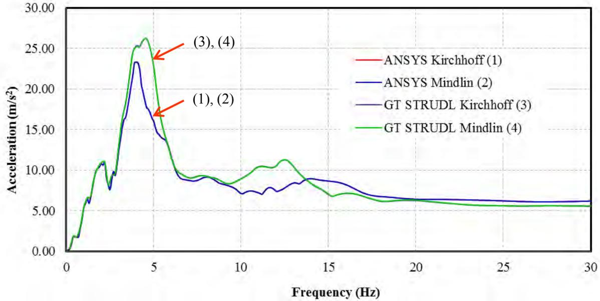
Figure 11. In-Structure X-Response Spectrum of El-Centro at Node 30776
