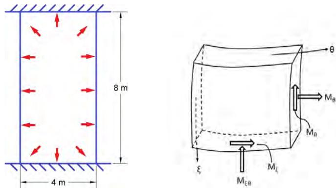
Figure 2. Cylinder Model with Associated Coordinate System
