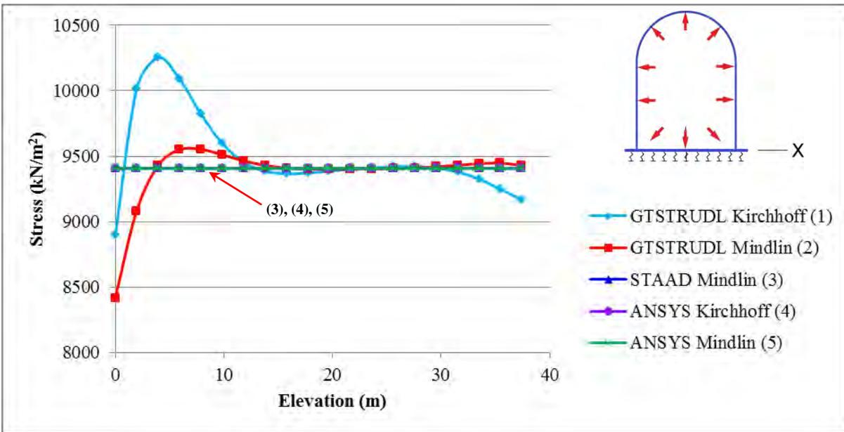
Figure 8. Middle Surface Vertical Stress at Various Containment Elevations
