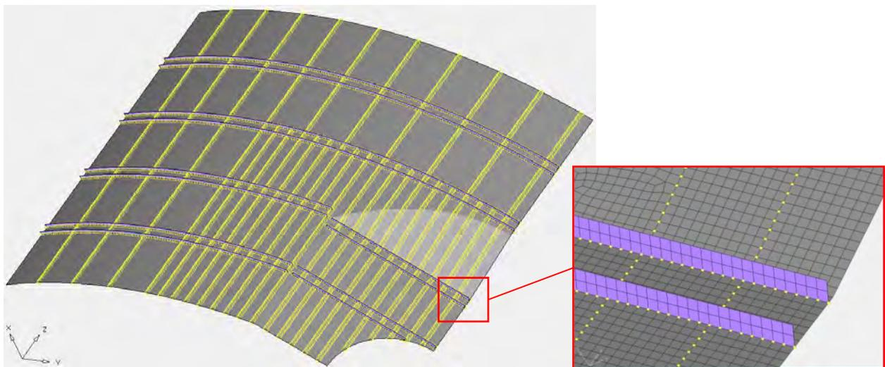
Figure 4. Liner FE-model with connectors highlighted in yellow and horizontal stiffeners modeled with shell elements.
