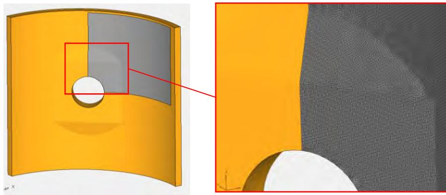
Figure 3. Position of local liner model (level 2).
