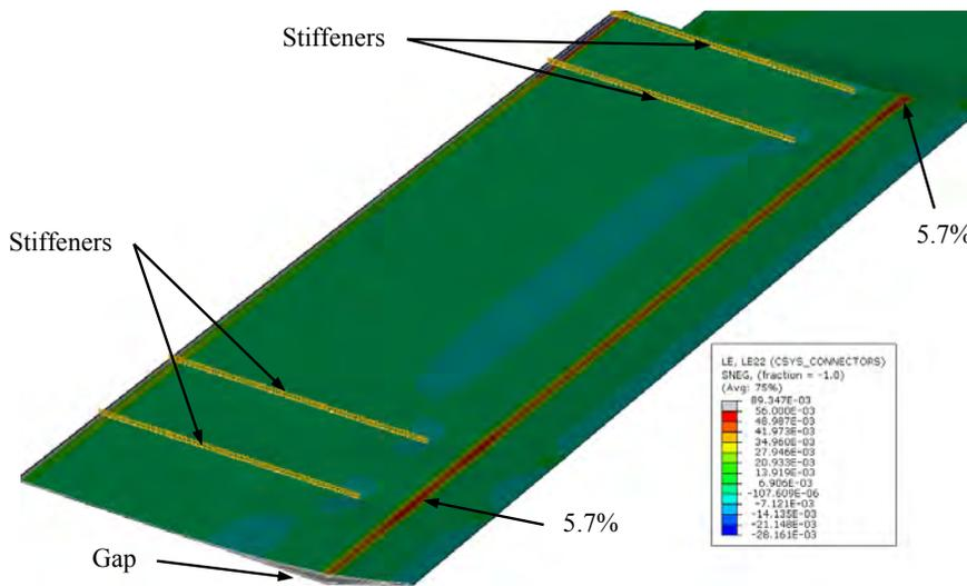
Figure 11. Detailed liner model, strain on liner inside at 1.29 MPa (3.3 pd) in hoop direction.
