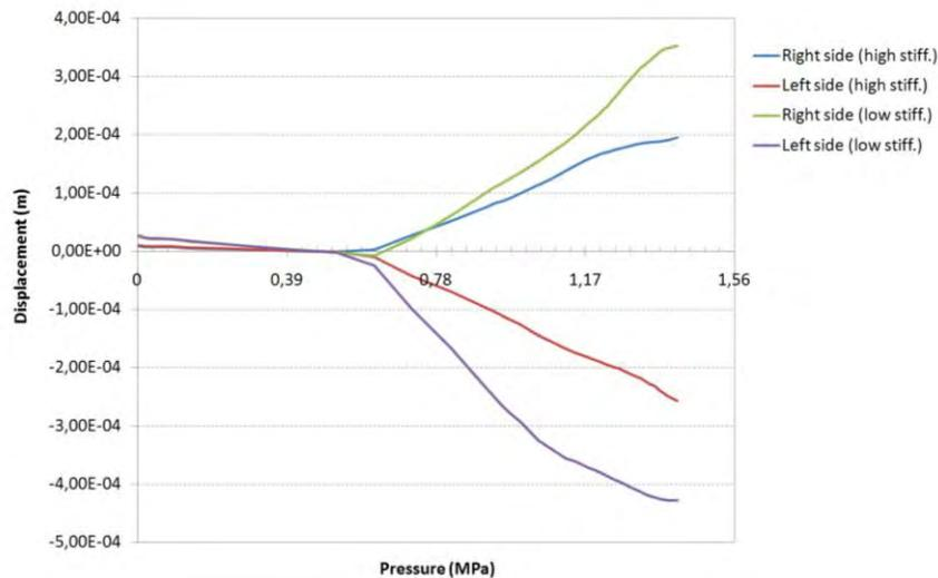
Figure 8. Liner anchor shear displacement near to vertical bend line (both sides of bend line at around level +5500).
