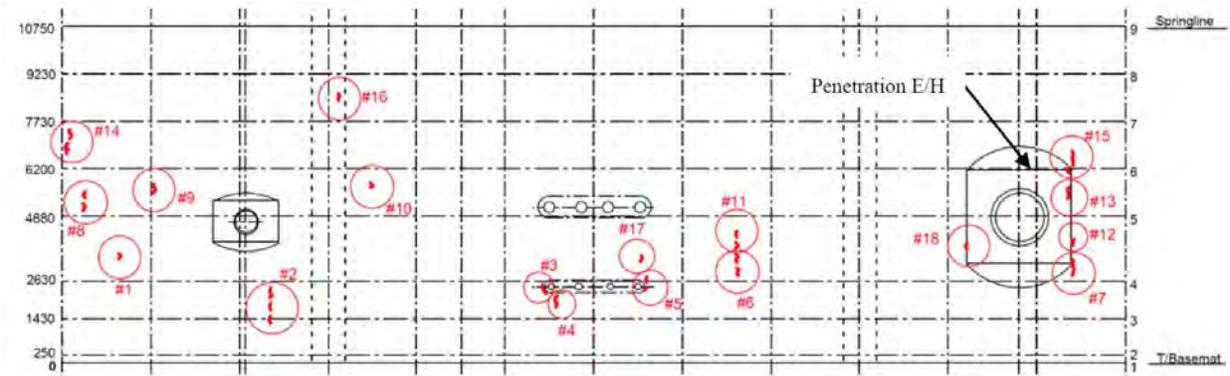
Figure 1. Stretched-out sketch, detected tears in the liner (Hessheimer M.F., 2003).
