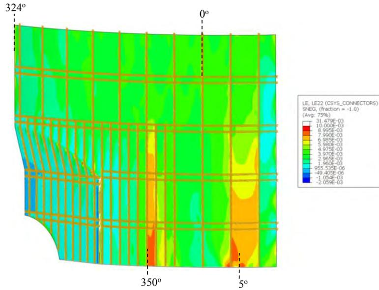
Figure 7.10 Liner strain at 1.29 MPa (3.3 pd) in hoop direction.
