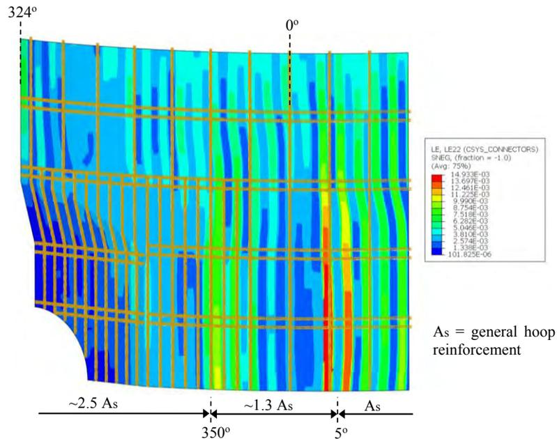
Figure 9 Concrete inner surface, strain at 1.29 MPa (3.3 pd) in hoop direction.
