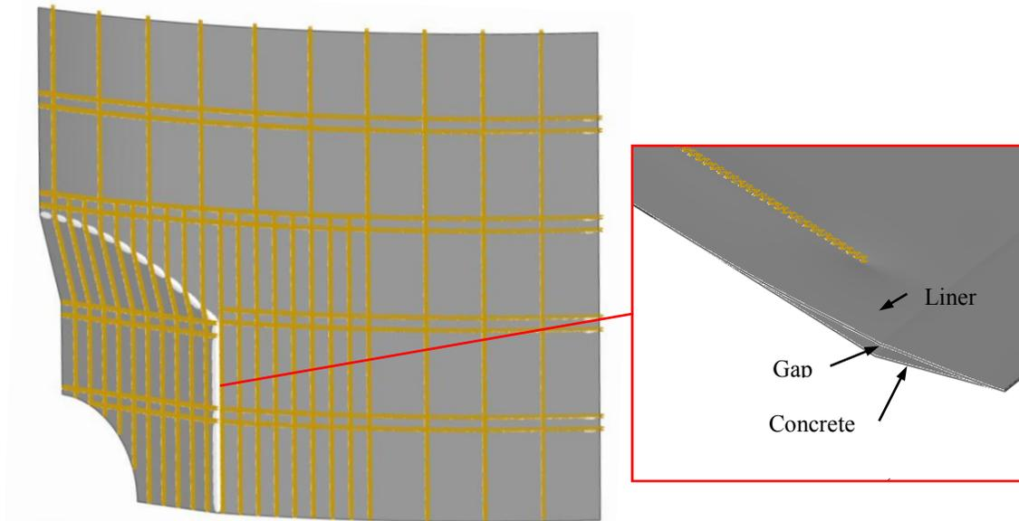
Figure 7. Concrete inner surface, separation between concrete and liner at 1.29 MPa (3.3 pd) in E/H region. White regions indicate where the liner has separated from the concrete.
