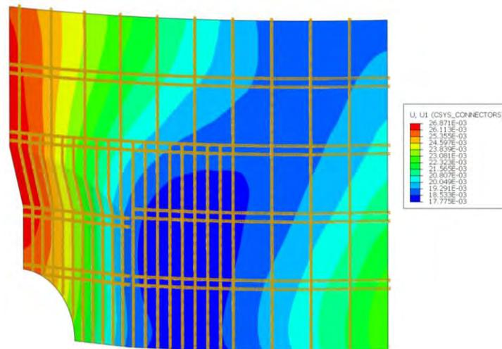
Figure 6. Concrete inner surface, radial displacement at 1.29 MPa (3.3 pd) in E/H region.
