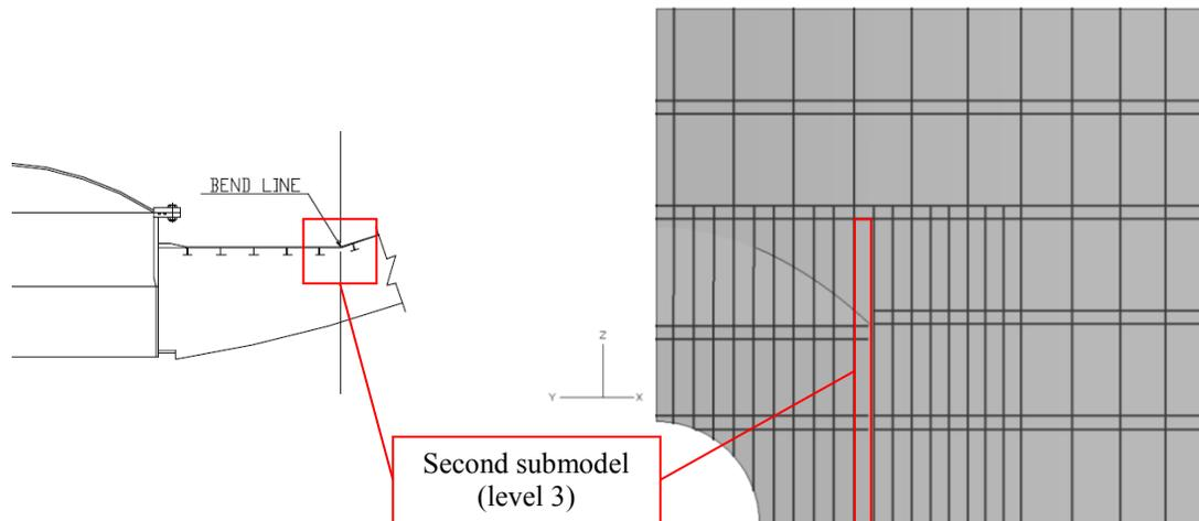
Figure 5. Left, excerpt from liner drawing in Hessheimer M.F. et al. (2003) showing a horizontal section through the E/H. Right, local liner model (level 2), where the location of the detailed liner model (level 3) is indicated.
