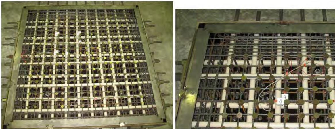
Figure 2. Test specimen with T-headed bars as shear reinforcement
