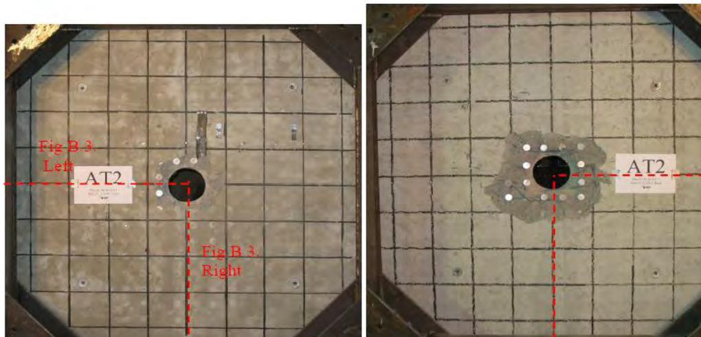
Figure 4. Test specimen with T-headed bars after the test (left-front face, right-rear face)
