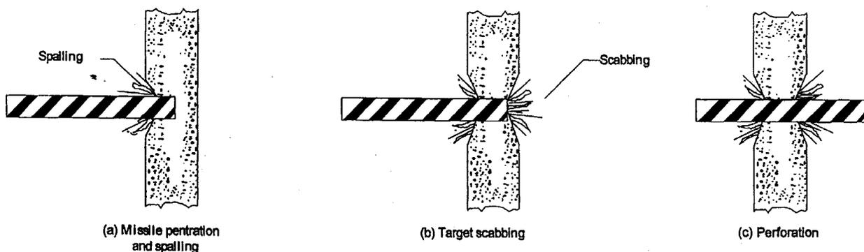
Figure 1. Sequence of Target Local Damage Due to Missile Impact, DOE (1996)
