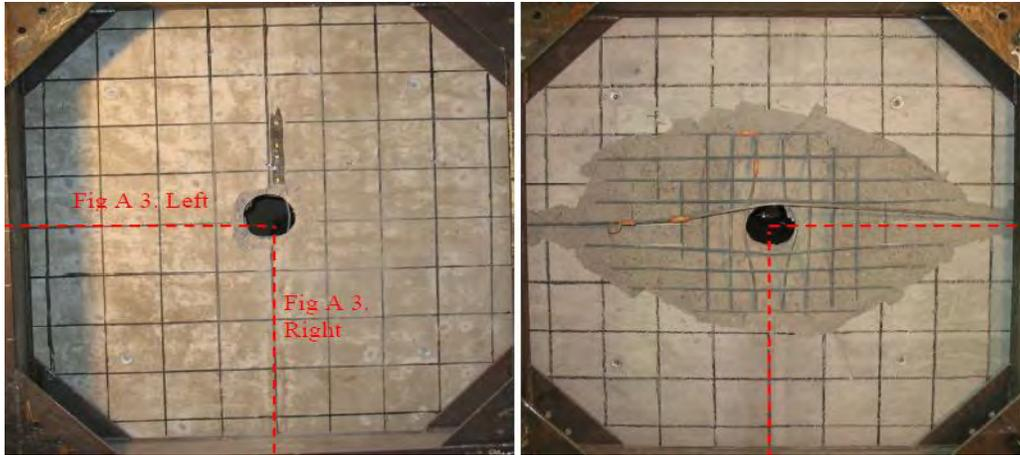
Figure 3. Test specimen without T-headed bars after the test (left-front face, right-rear face)
