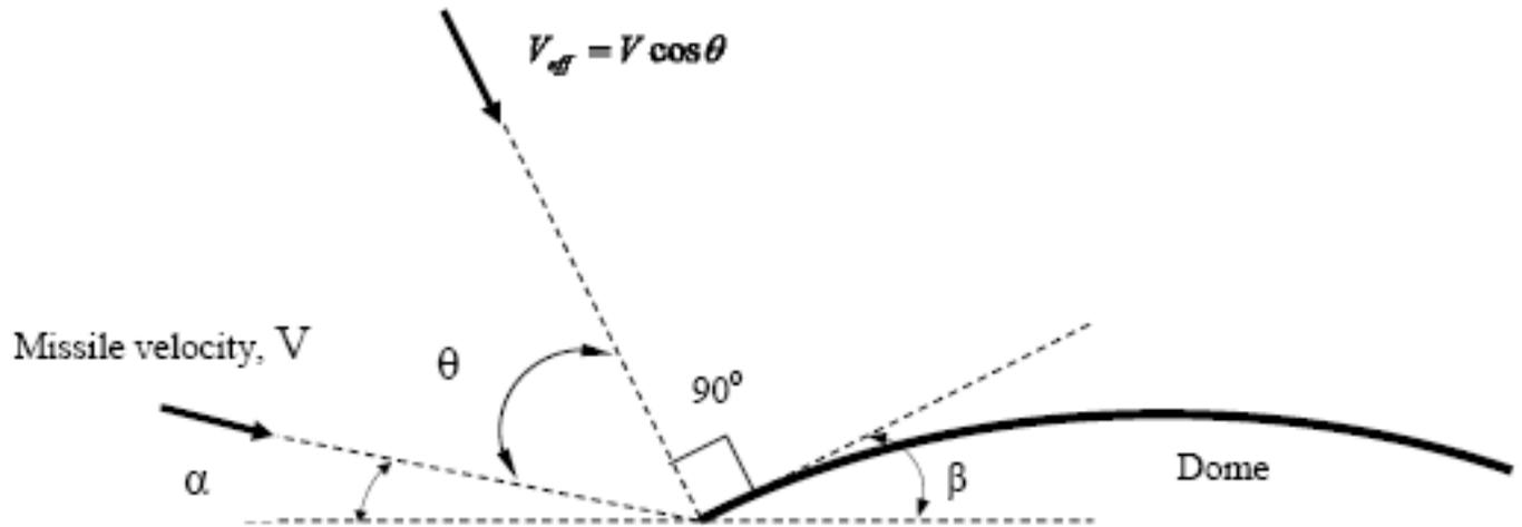
Figure 5. Schematic view of the missile hit the dome at angle  $\alpha$
