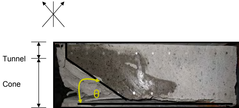
Figure 4 Horizontal cut in the middle of the slab without transverse reinforcement
