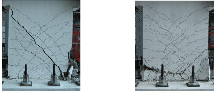
(a) RC specimen at 2.25% drift (b) R-SFRC specimen at 3.5% drift
