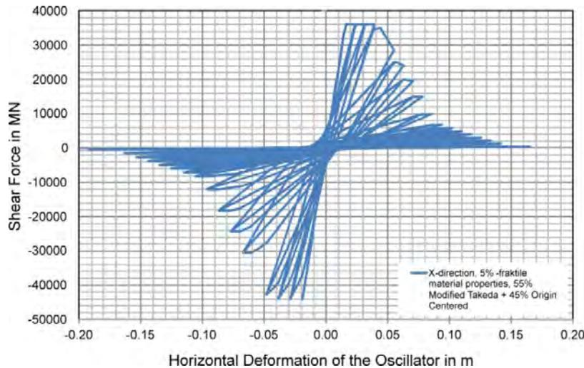
Figure 9. Hysteresis in X-direction using the 5 % fractile Value of Material Properties.
