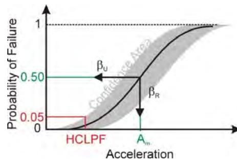
Figure 1. Seismic Fragility: Terms..
