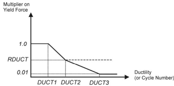
Figure 8. Model for ductility dependent on stiffness-drop according to Ruaumoko (Carr 2004).
