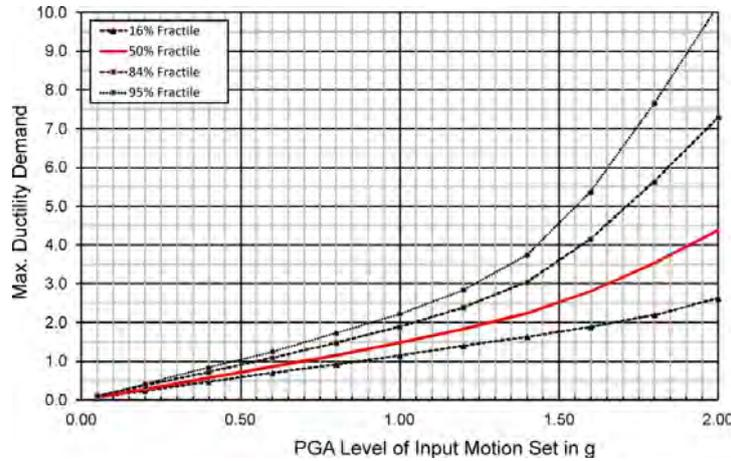
Figure 11. : Incremental dynamic analysis for representative oscillator with characteristic material values.
