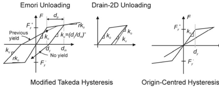
Figure 7 Used hysteresis rules for the non-linear dynamic analysis.
