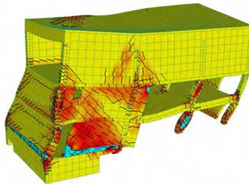
Figure 3. Deformation of the structure during a pushover-analysis.
