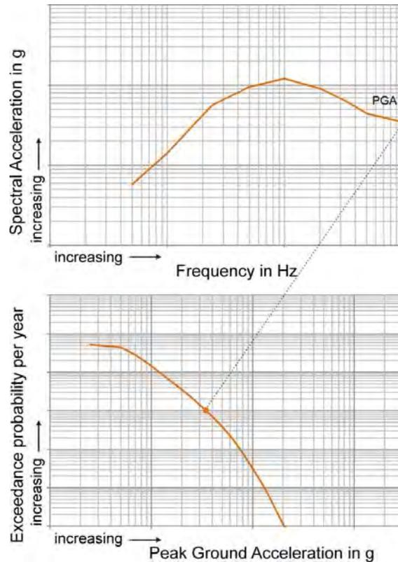
Figure 5. Uniform Hazard Spectrum and Hazard Curve (PGA: Peak Ground Acceleration).
