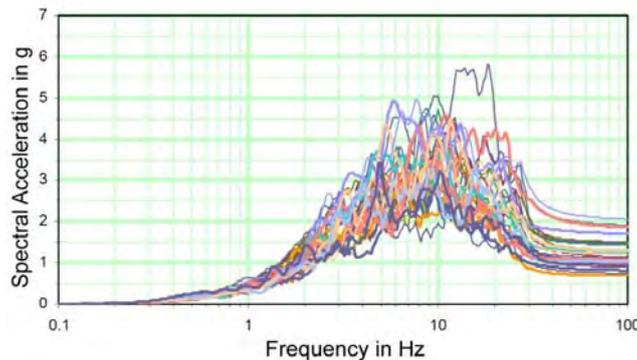
Figure 11. Individual Spectra of the different Acceleration-Time-Functions.
