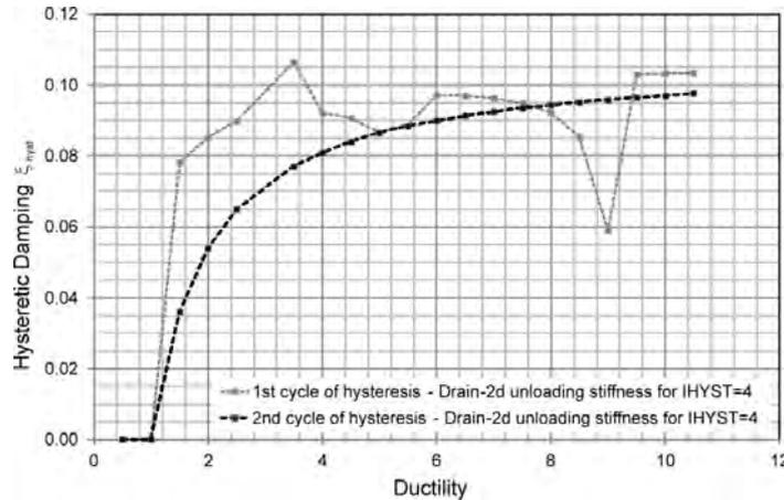
Figure 10. Hysteretic damping of the oscillator.
