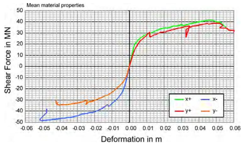
Figure 4. Pushover-curve based on mean material properties.
