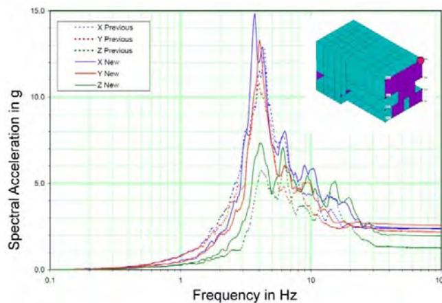
Figure 6: Floor Response Spectra in the upper part of the building
