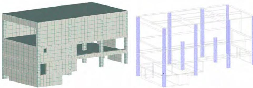
Figure 2. Mesh of the Finite-Element-Model used (above) and visualization of the reinforcement modeled in the columns (bottom).
