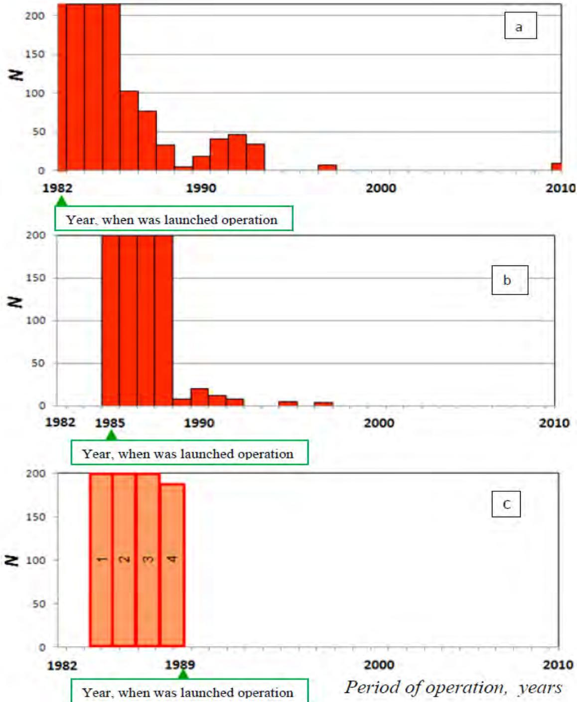
Figure 4. The results of the application of compensatory measures for existing nuclear power plants. Pipelines DN800 MSP RBMK-1000, SmNPP. The vertical axis - the number of detected and repaired defects, N.
