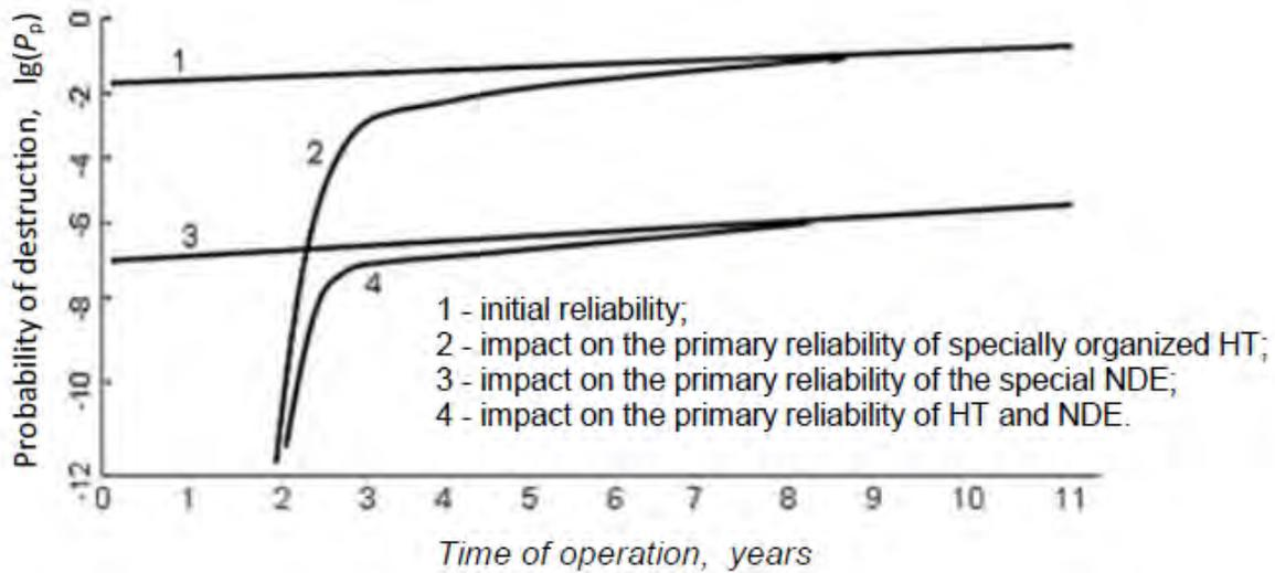
Figure 2. Change in the probability of rupture of the main pipeline of the reactor VVER-440 depending on the activities
