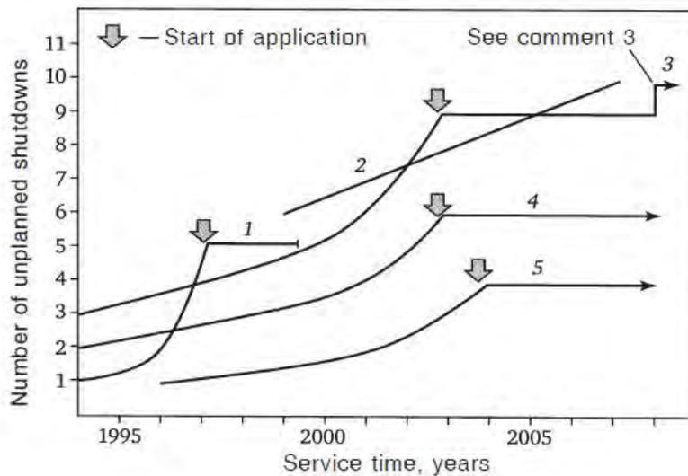
Figure 1. Dynamics of unplanned shutdowns before and after the application of the RD EO-0552-2004(1-Unit 2 BalNPP; 2-Unit 1 KaNPP; 3-Units 3 and 4 NVNPP; 4-Units 1 KolNPP; 5-Unit 2 KolNPP).
