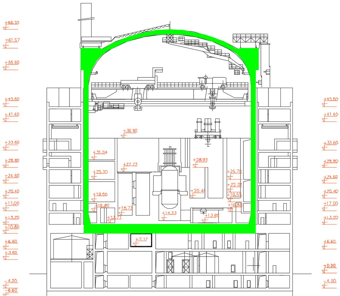
Figure 1. Section view of VVER1000 Reactor building, concrete containment is marked by green filling
