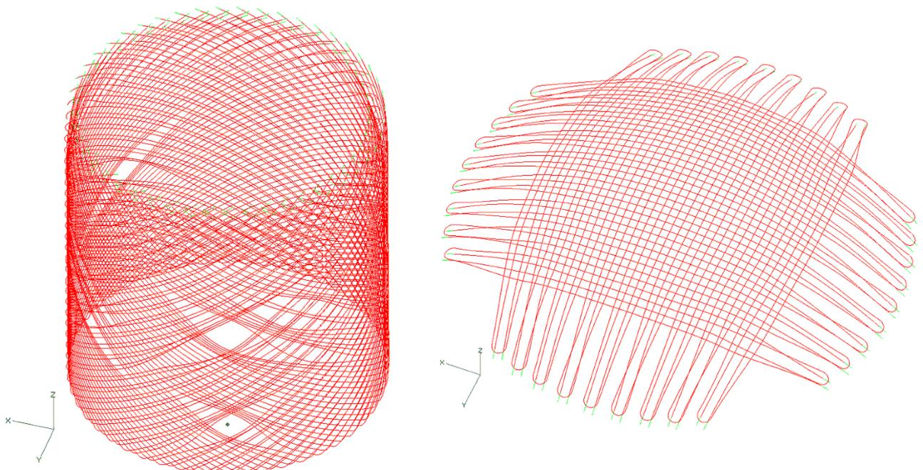
Figure 3. Layout of cylindrical and dome tendon ducts
