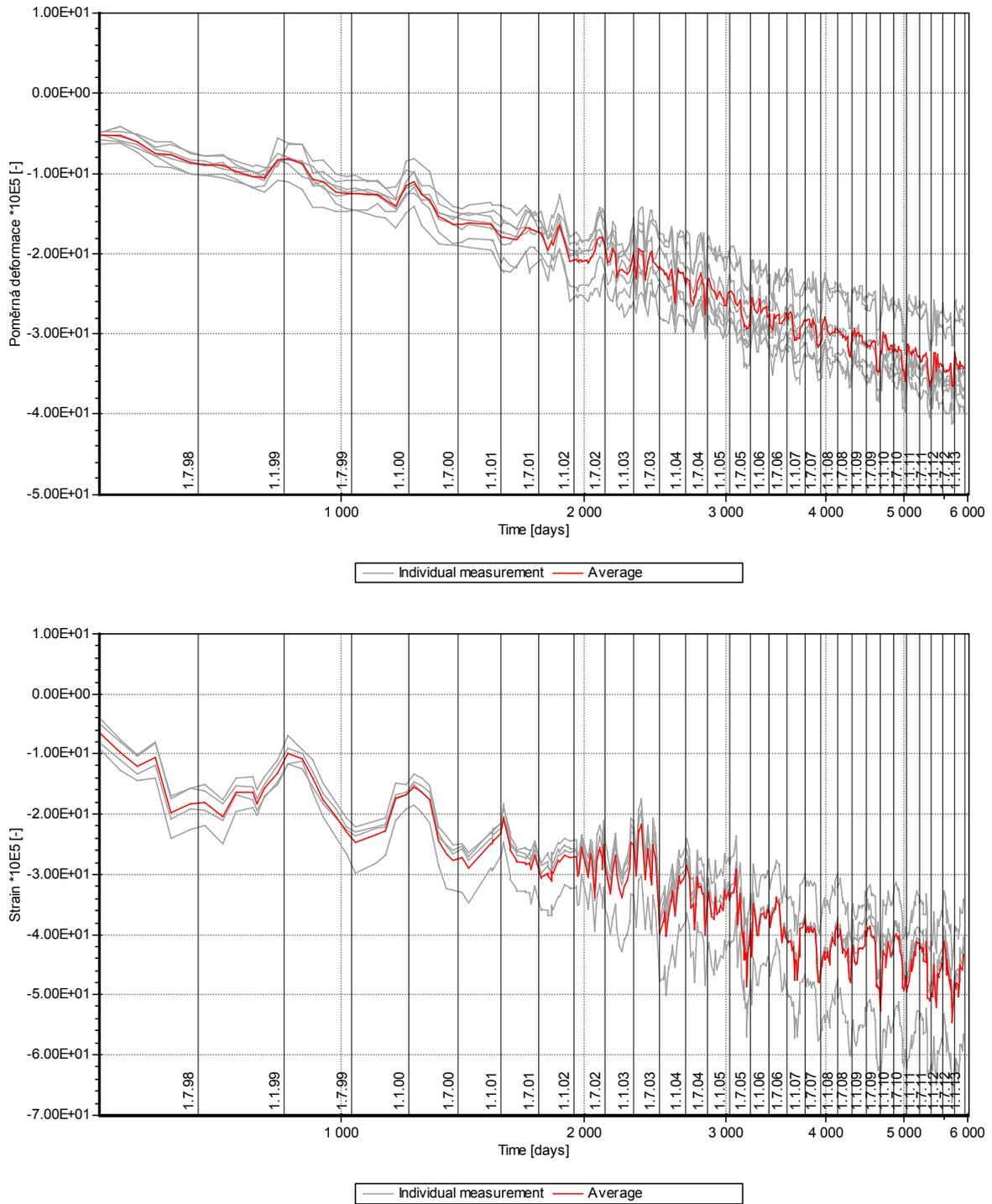
Figure 8. Unit 2 - Measurement of vertical strain in the middle of cylinder height and in the middle of dome during operation
