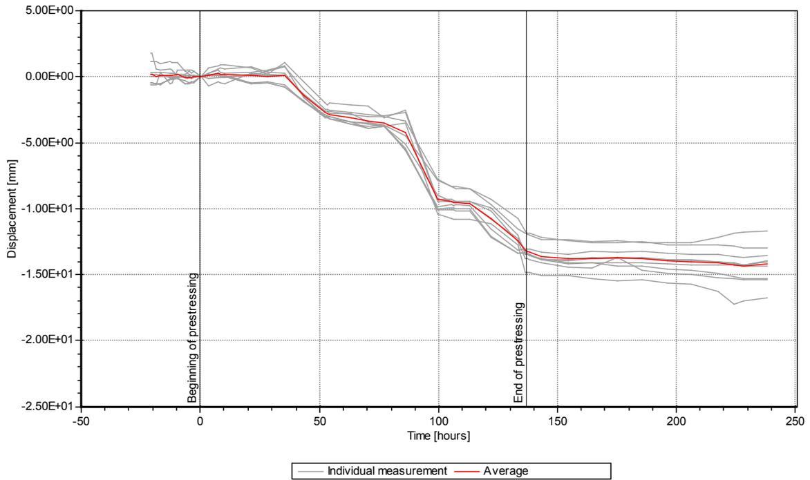
Figure 6. Unit 2 - Measurement of horizontal displacements in the middle of cylinder height during prestressing
