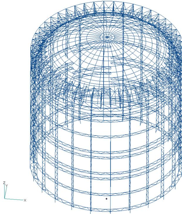
Figure 4. Layout of steel structure of formwork
