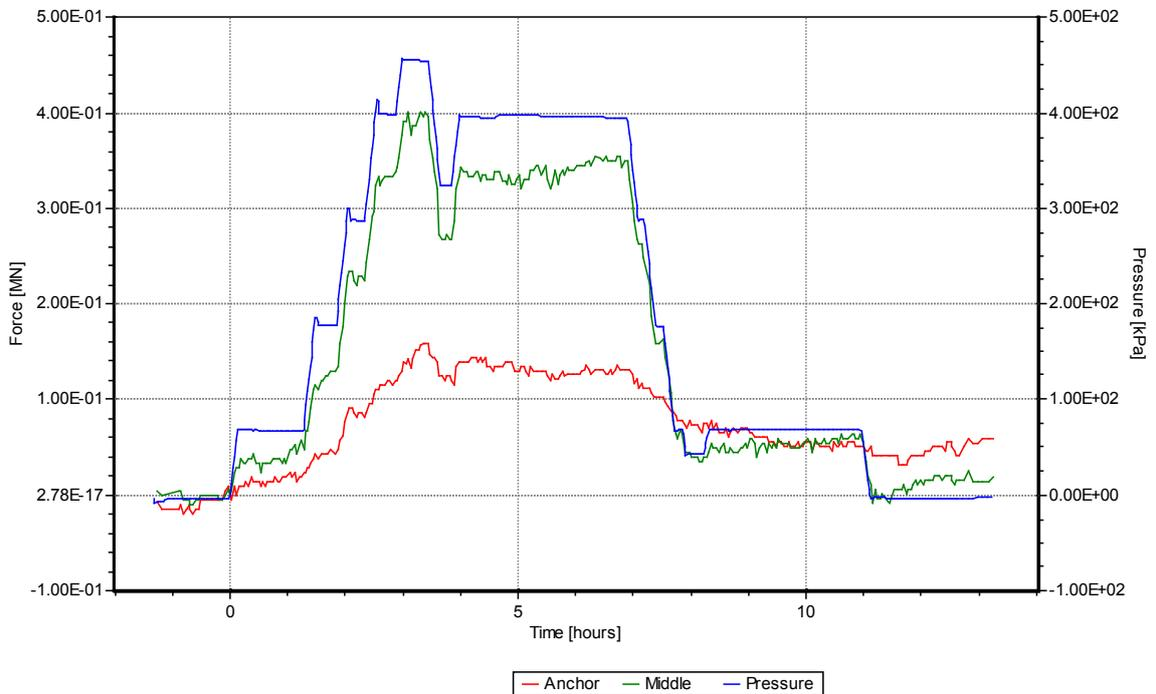
Figure 7. Changes of prestressing force along cylindrical tendon length during SIT at Unit 2
