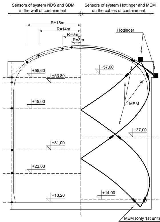
Figure 5. Distribution of sensors on the containment structure
