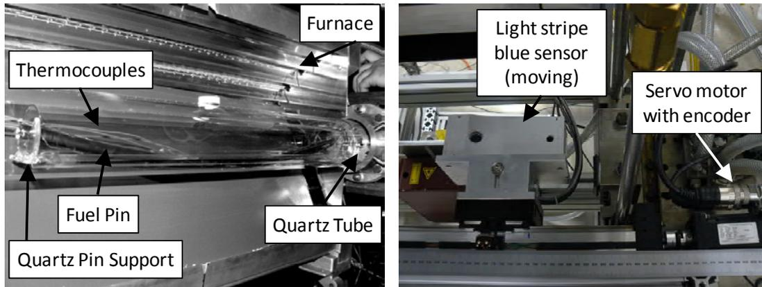
Figure 2. Experimental set-up for a high temperature fuel sag test using an infra-red parabolic furnace.
