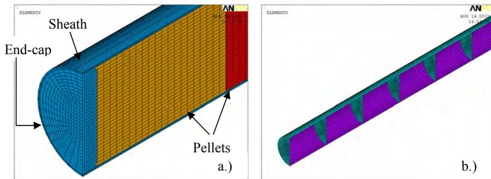
Figure 8. ANSYS model geometry: a.) Finite element mesh used; b.) Pellet-to-pellet and pellet-to-sheath contact elements.
