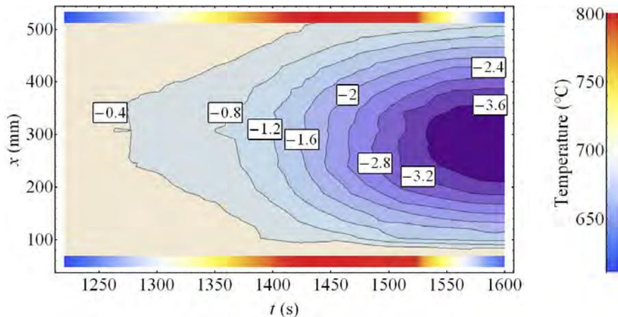
Figure 6. Labeled contour plot of vertical deflection  $\Delta z_0$  (mm) showing dependence on time, temperature, and axial position, from experimental analysis, during the first temperature cycle to 800°C.
