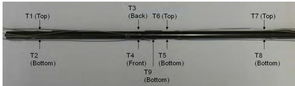
Figure 1. Thermocouple locations for the fuel pin sag test.
