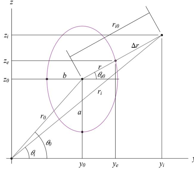
Figure 4. Geometric sketch with symbols used for fitting ellipses to set of data points judged to be on the fuel-pin surface.
