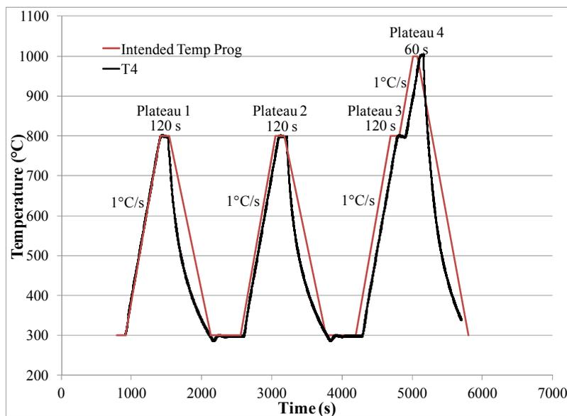
Figure 3. Planned temperature program and measured sheath temperature near the fuel-pin mid-plane.
