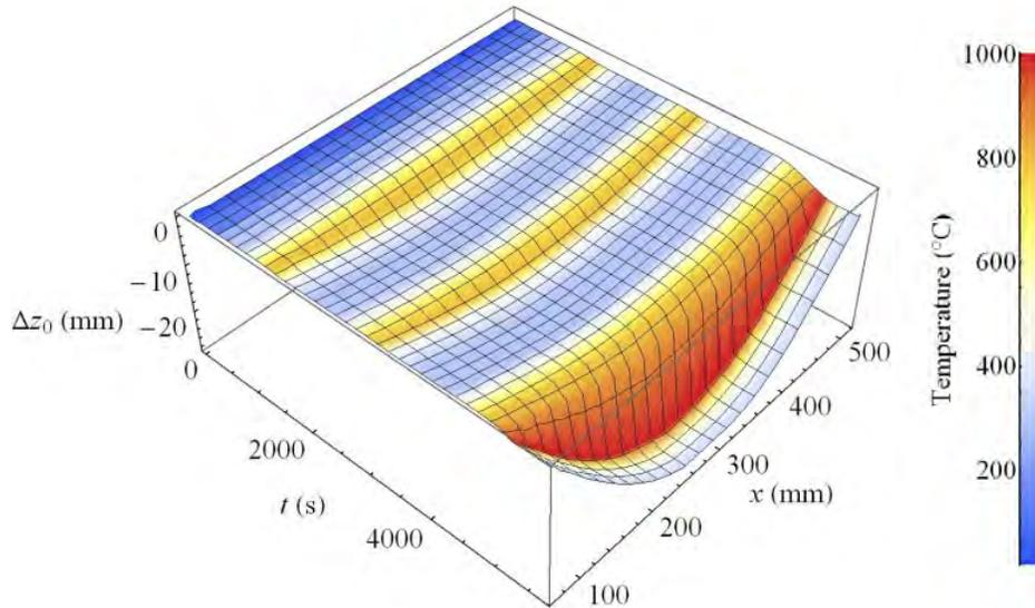
Figure 7. Vertical deflection, from experimental analysis, showing dependence on time, temperature, and axial position.
