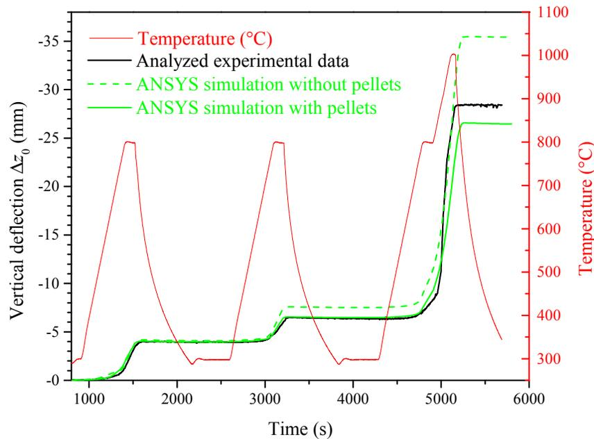
Figure 9. Experimentally measured vertical deflection near mid-plane of the unsupported fuel-pin span ( $x = 282$  mm) compared with ANSYS-based simulations.
