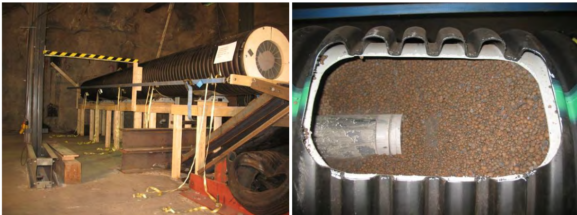
Figure 3. Test setup where shock absorber diameter was 600 mm and canister diameter 112 mm.
