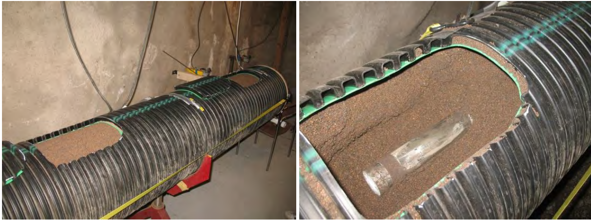
Figure 2. Test setup where shock absorber diameter was 400 mm and canister diameter 63 mm.
