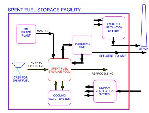
Figure 1. Flow sheet of SFSF
