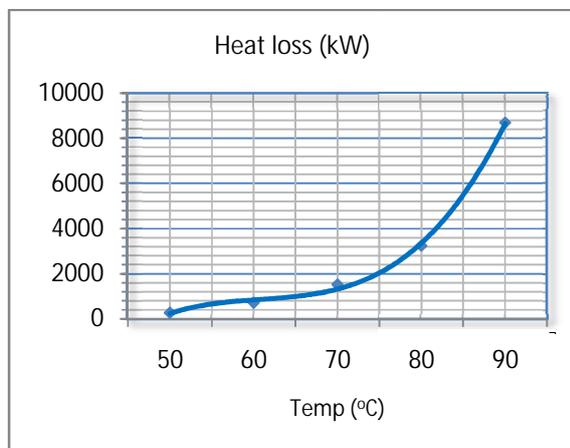
Figure 5. Heat loss Vs pool water temperature
