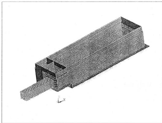
Figure 3. 3-D FEM model of fuel pool
