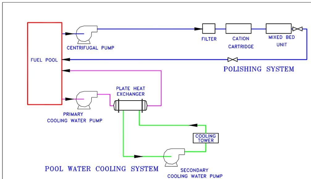
Figure 2. Schematic of pool water cooling system and polishing system
