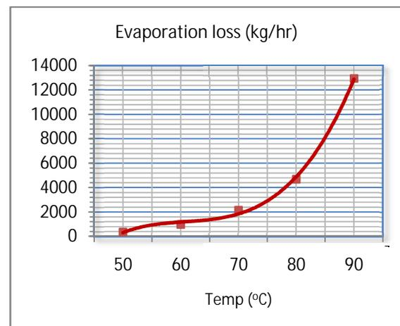
Figure 6. Evaporation loss Vs pool water temperature
