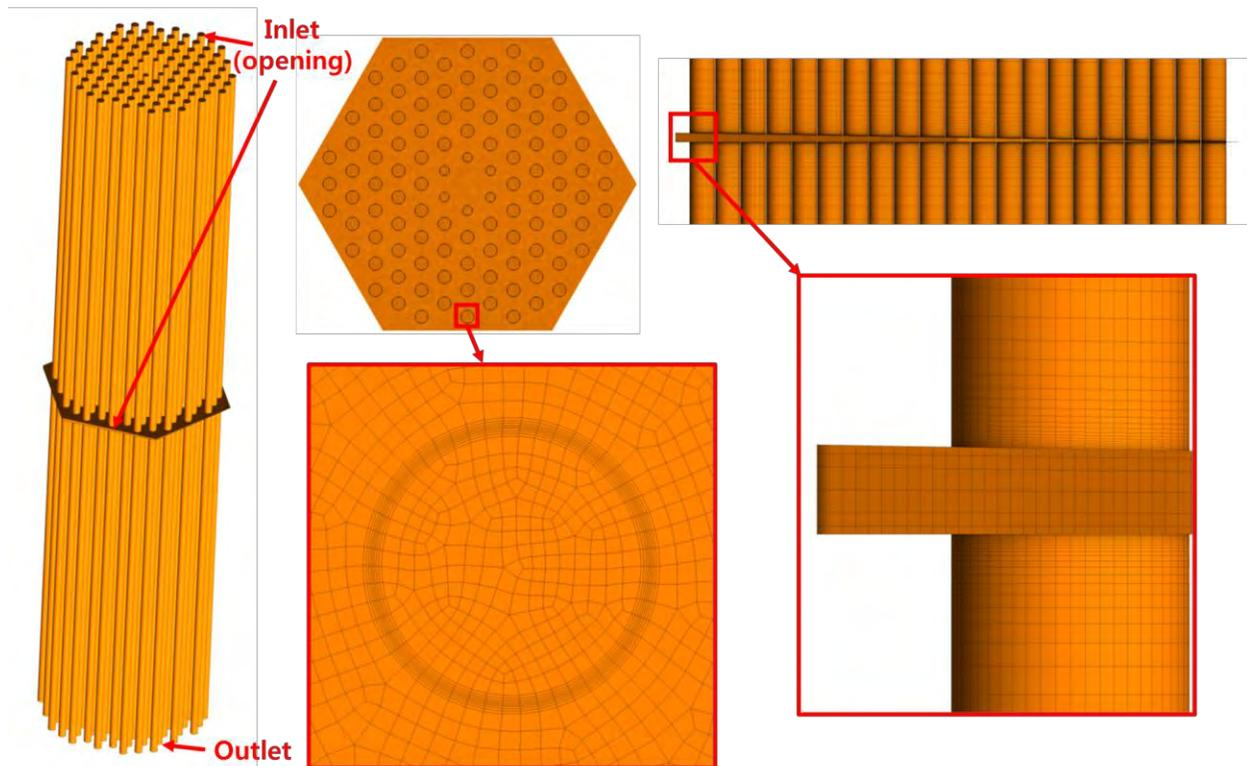
Figure 4. Computational domain and mesh structure
