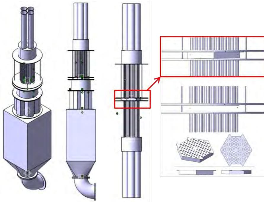
Figure 2. Design of the experimental apparatus and cross gap
