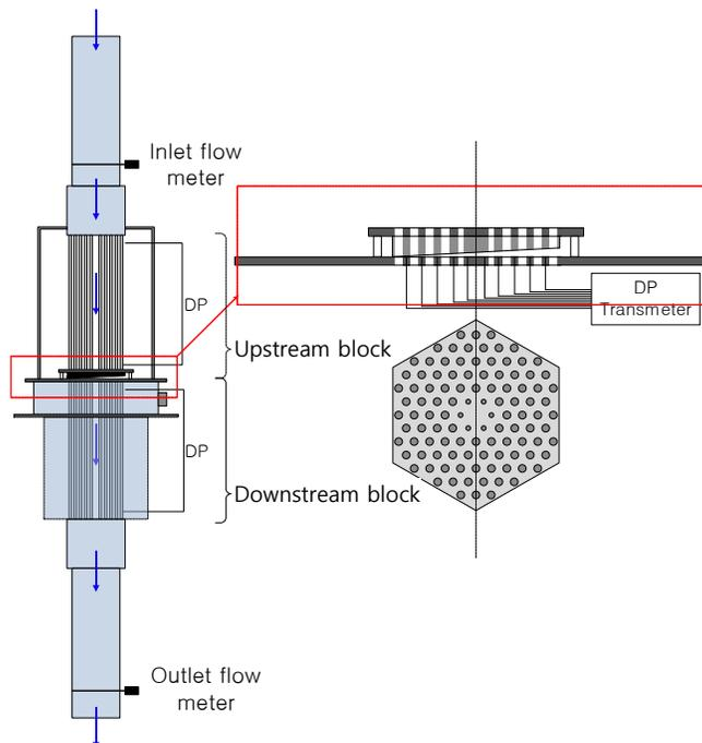
Figure 1. Schematic view of experimental apparatus
