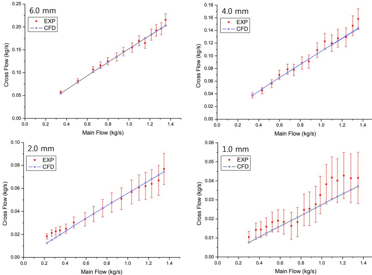
Figure 5. The cross flow rate to the total flow rate
