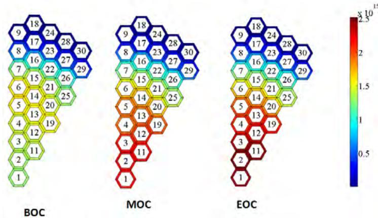
Figure 7 – Flux at mid-core (flux node 5, z = 59.2in) for the beginning, middle, and end of cycle.
