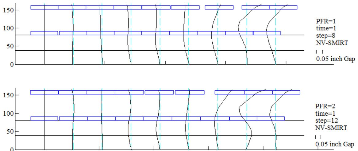
Figure 9 Duct deformations for radial row showing exaggerated duct deflections and load pads (blue rectangles) at P/F=1 (top) and P/F=2 (bottom).
