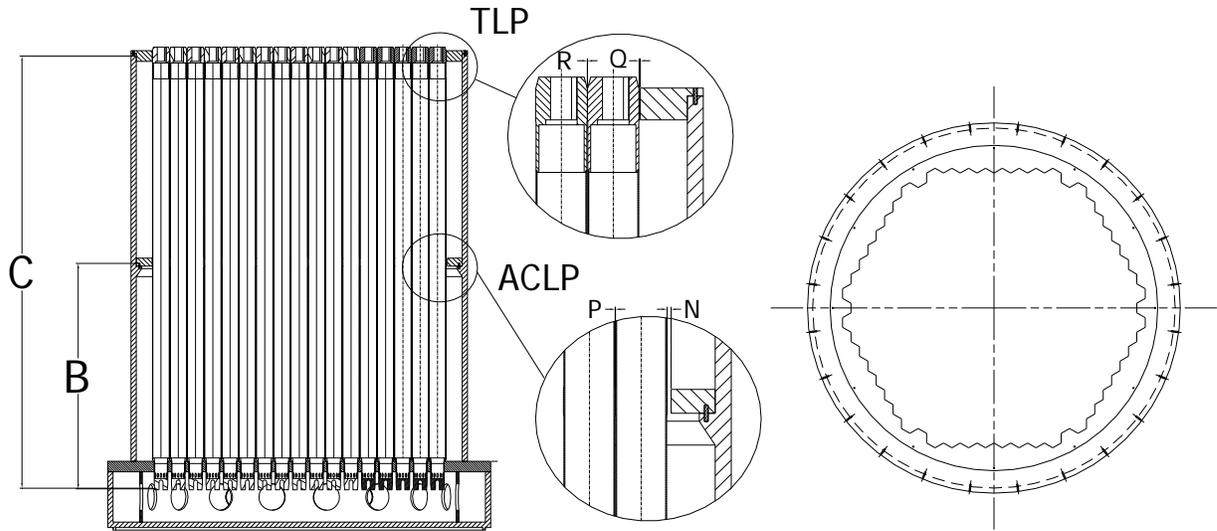
Figure 4 – Details of the core restraint system.
