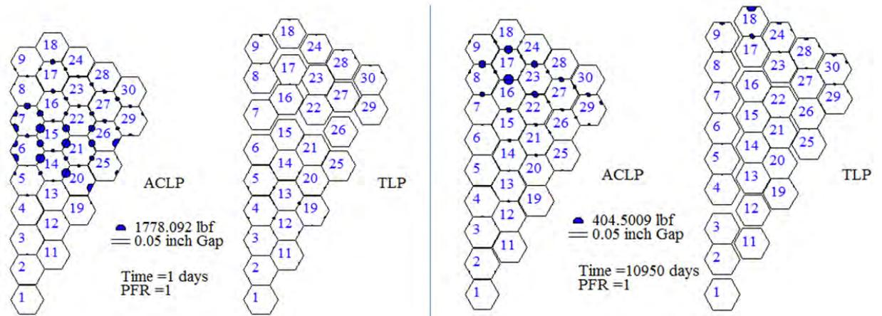
Figure 10 Exaggerated displacements and contact forces at the ACLP and TLP for days 0 (left) and 10950 (right) at P/F=1.
