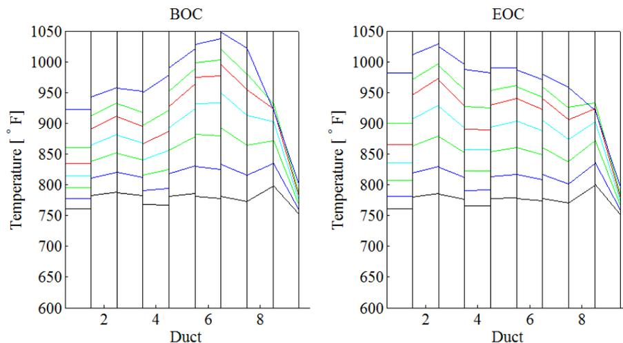
Figure 6 – Radial temperature distribution across ducts 1-9 for BOC and EOC. Colors correspond to different axial points along the duct.
