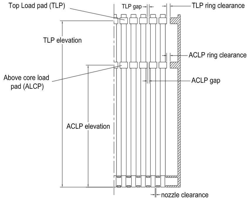
Figure 1 – Schematic representation of core restraint system components and important dimensions.
