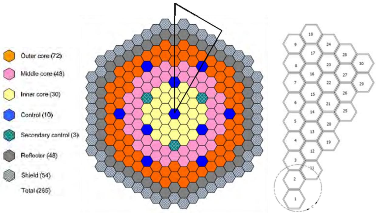
Figure 5 – AFR100 non-vented core layout (from (Grandy, et al., 2013)) and 30 degree sector used in NUBOW analysis.
