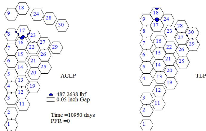
Figure 8 – Residual inelastic deformations and resulting contact loads at refueling temperatures at EOC.
