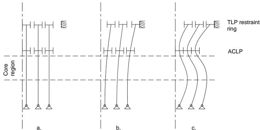
Figure 2 – Schematic illustration of limited free bow core restraint concept.
