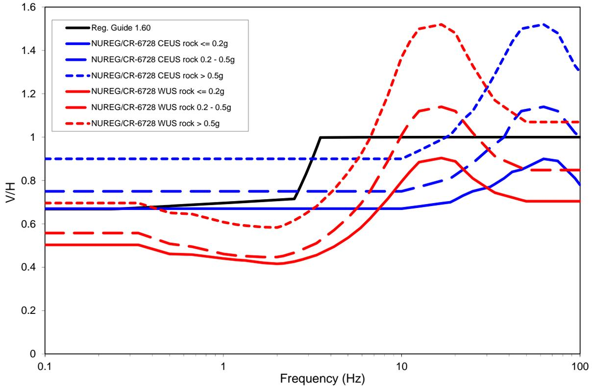
Figure 5. V/H Ratios from Reg. Guide 1.60 (NRC, 1973) and NUREG/CR-6728 (McGuire et al., 2001).
