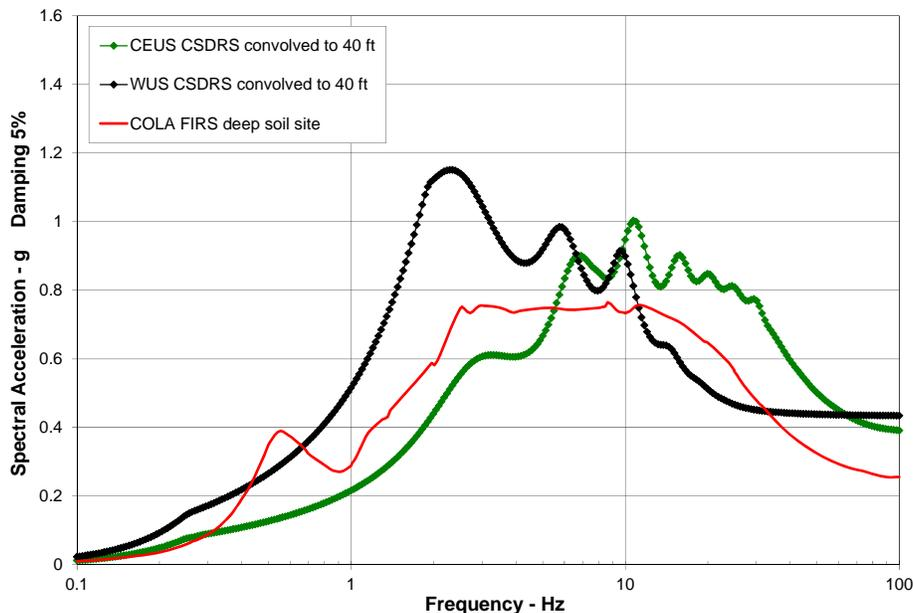
Figure 4. Comparison of CSDRS Convolved to Depth of 40 ft. with a Selected COLA FIRS.
