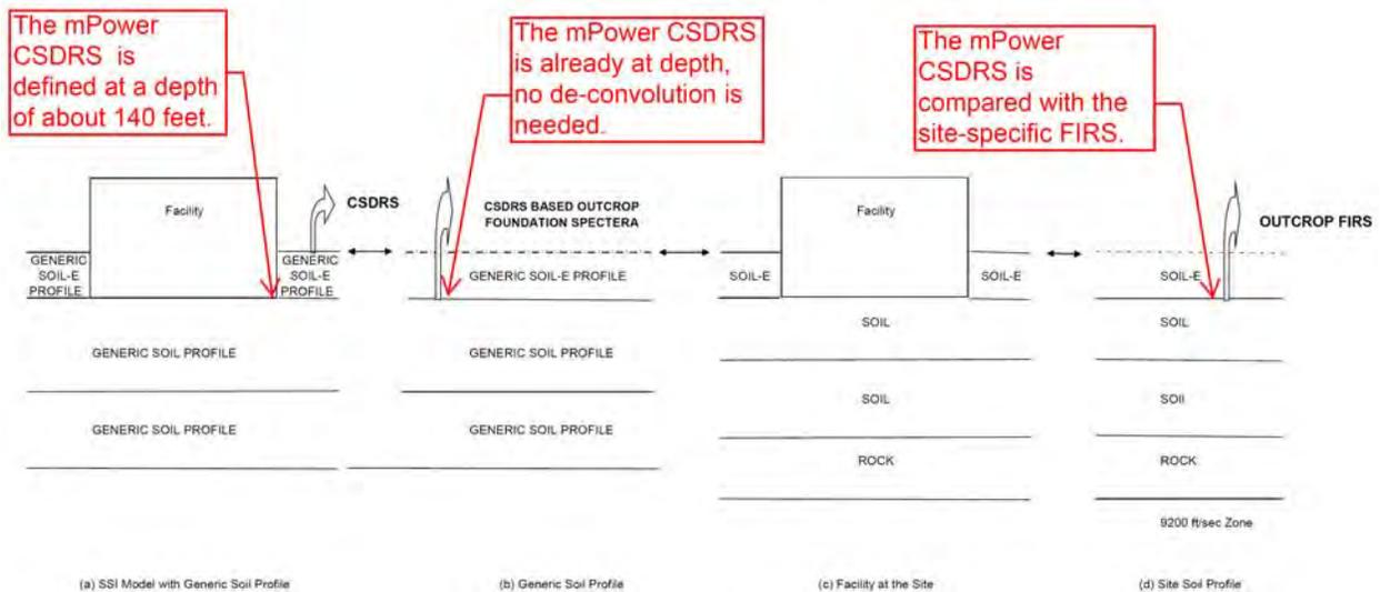
Figure 3. Comparison of CSDRS with FIRS – Nuclear Energy Institute (2009).
