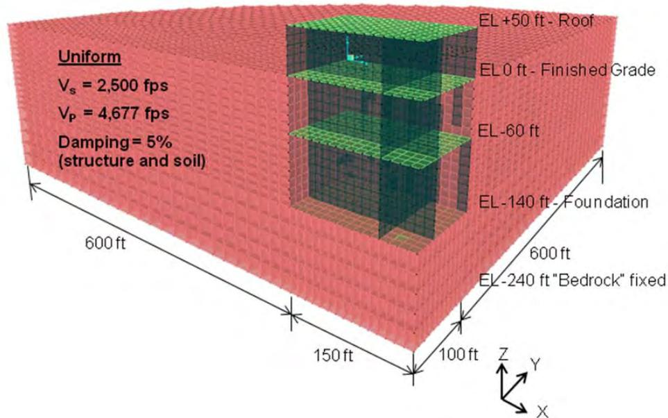
Figure 6. Model Geometry used for Global Validation.
