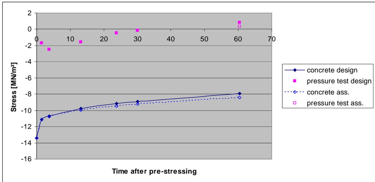
Figure 7: Concrete stress for the cylindrical part in horizontal direction
