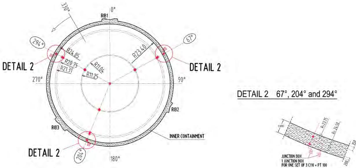
Figure 3: Location of measurement devices in cylindrical part and in dome
