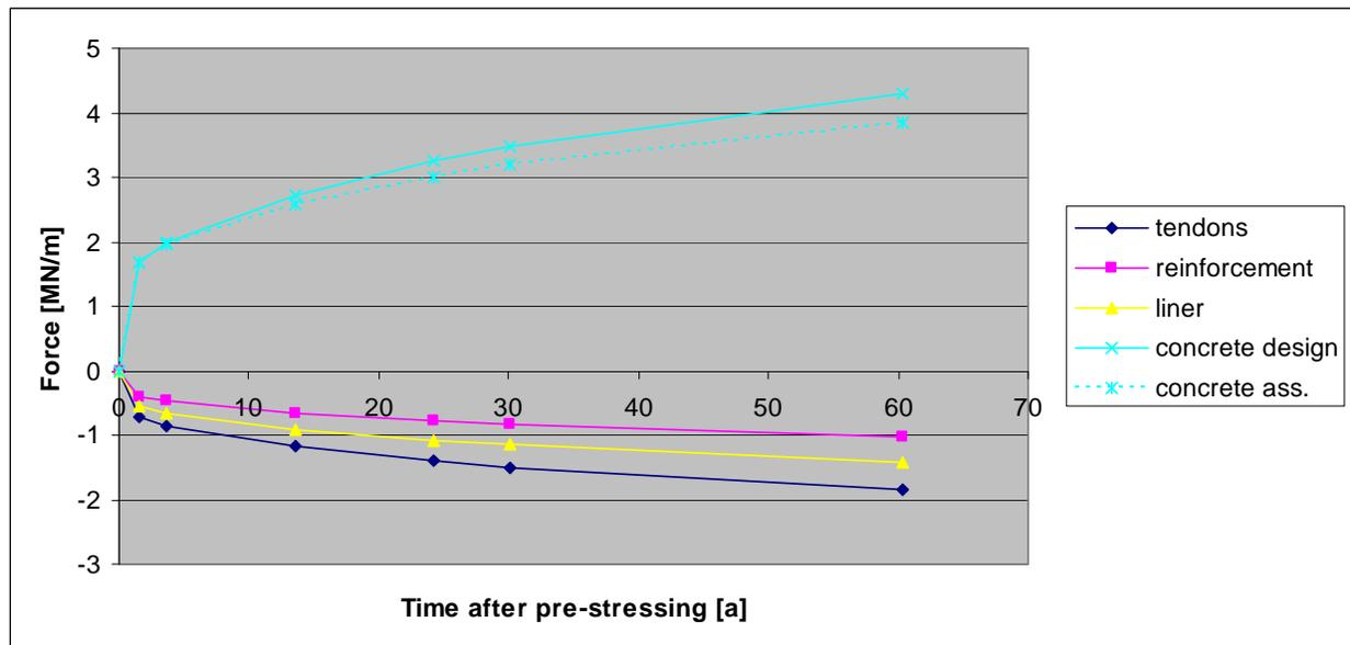
Figure 6: Force balance for the cylindrical part in horizontal direction
