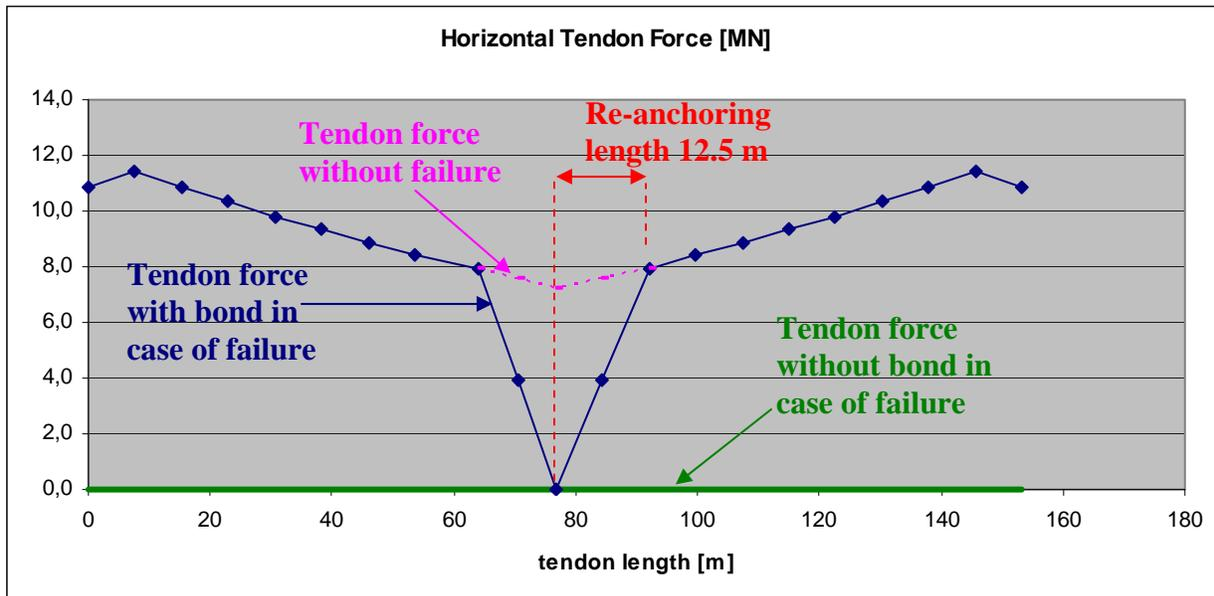
Figure 4: Tendon force and re-anchoring length
