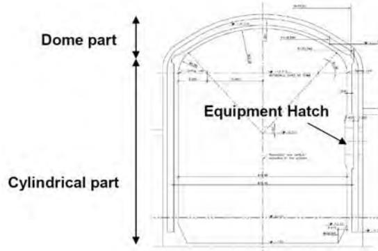
Figure 1: Inner and outer containment of the EPR™
