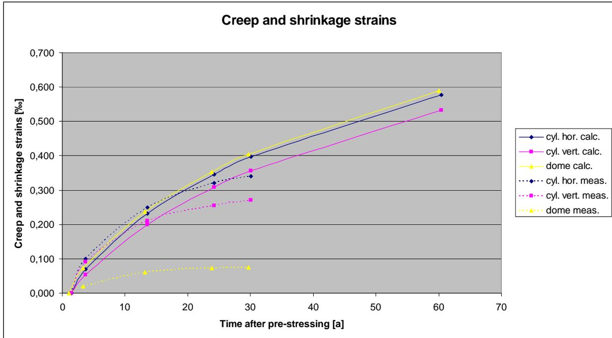
Figure 5: Calculated and measured creep and shrinkage deformations
