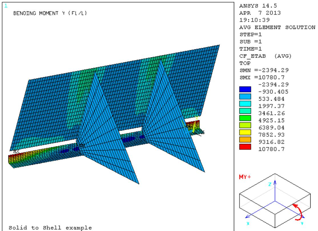
Figure 3 Example bending moment per unit length plot
