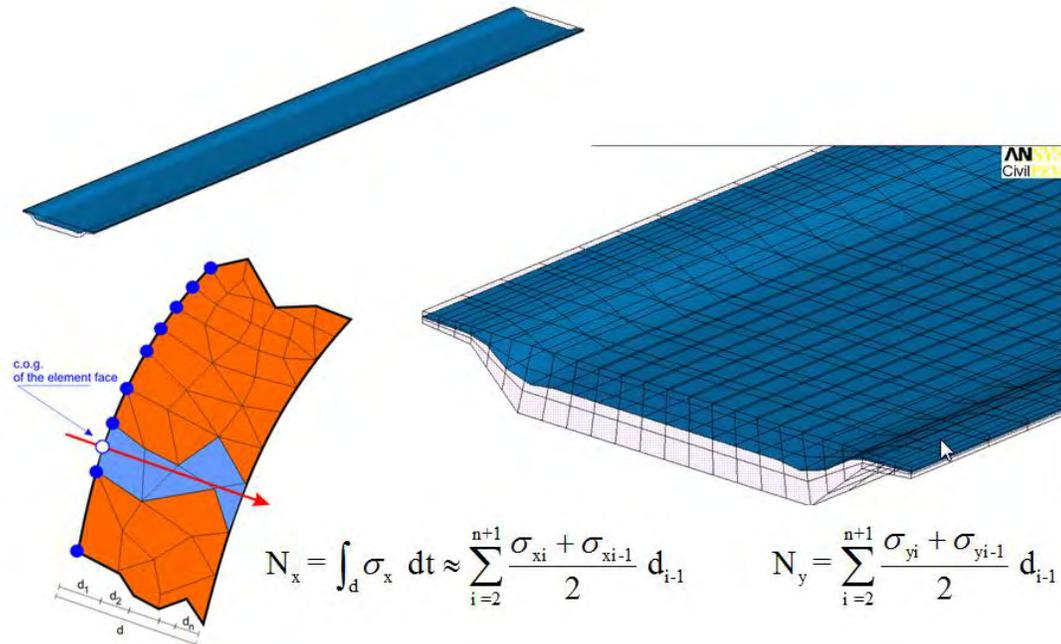
Figure 2. Pseudo shell element used to develop force and moments per unit length for code evaluation
