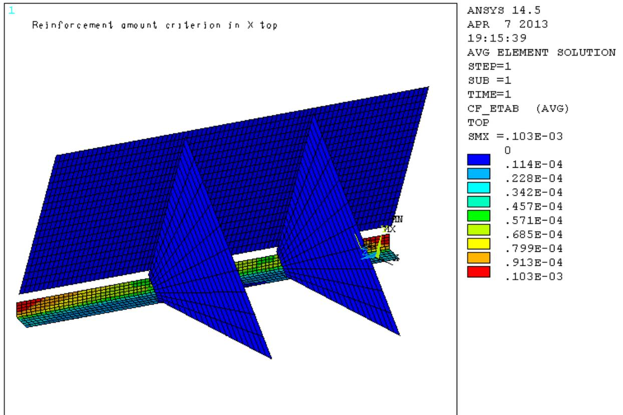
Figure 4 Example reinforcement ratio on the top shell surface per unit length
