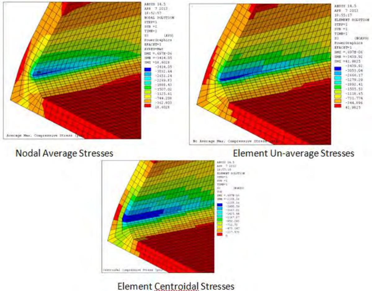
Figure 1. Example stress values including nodal averaged vs. unaveraged vs. element centroidal values
