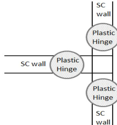
Figure 1 Typical T joint configuration in CIS      Figure 2 – Recommended failure mode for T-joints
