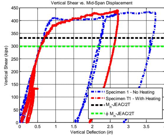
Figure 6 - Average load vs. average net mid-span deflection comparison of Specimen T1
