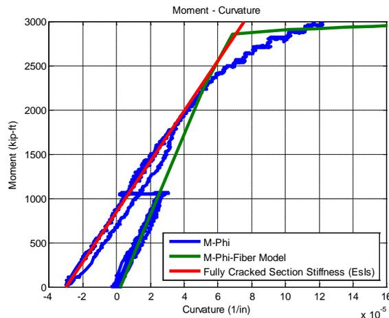
Figure 7 - Moment-curvature behavior of Specimen T1, zoom into initial loading stage
