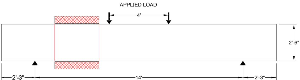
Figure 8 - Elevation View with Heaters of Specimen T2
