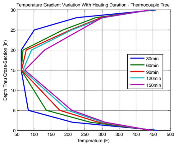
Figure 10 - Thru-depth temperature distributions obtained using the thermocouples on the thermocouple tree
