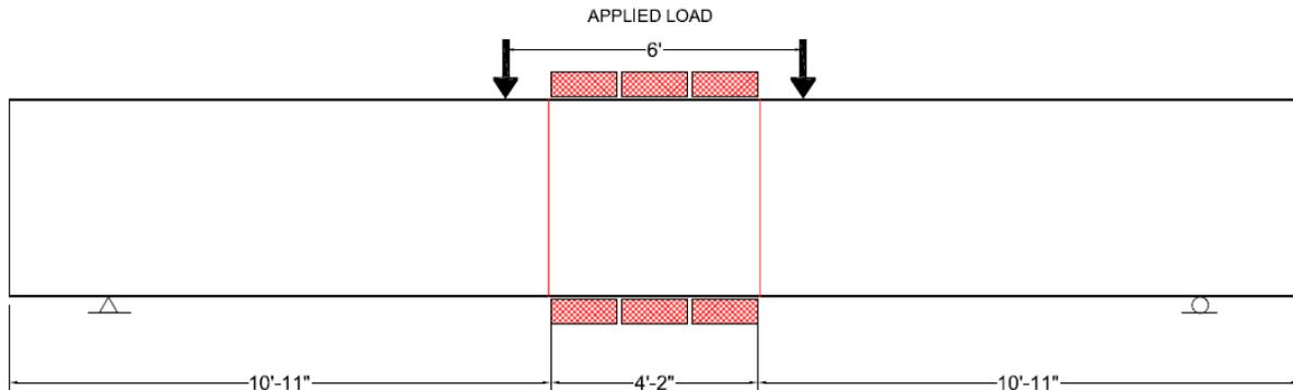
Figure 2 - Elevation View with Heaters of Specimen T1
