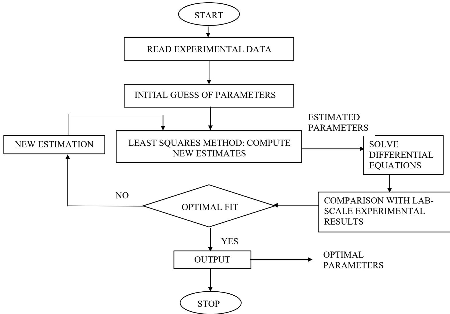
**Figure 2.** Flow chart for the estimation and optimization of kinetic parameters in the anaerobic co-digestion of swine manure and corn stover.
