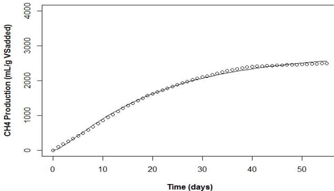
**Figure 5.** Simulation of methane generation in batch experiments using optimized values of kinetic parameters (○ experimental data; — model simulation).
