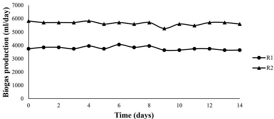
**Figure 2.** Daily biogas production in anaerobic reactors treating swine wastewater with untreated and lime-treated corn stover
