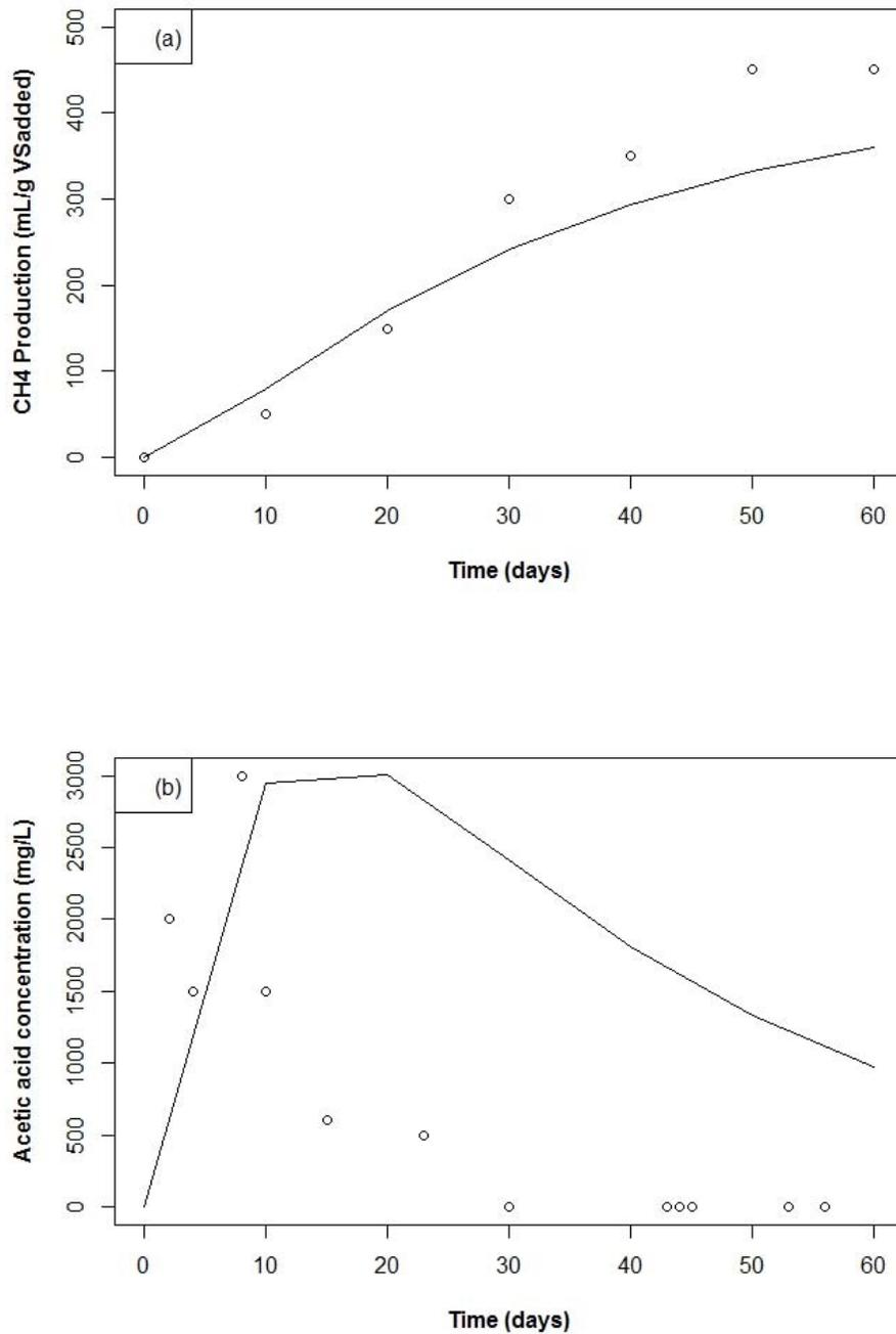
**Figure 6.** Simulation of methane yield and acetic acid concentration by proposed model in comparison with experimental data from Cuetos et al. (2011) (○ experimental data; — model simulation; the values of model parameter under mesophilic condition were converted from thermophilic calibrated parameter values based on the equation  $F(T) = e^{\theta(T-T_0)}$ ).
