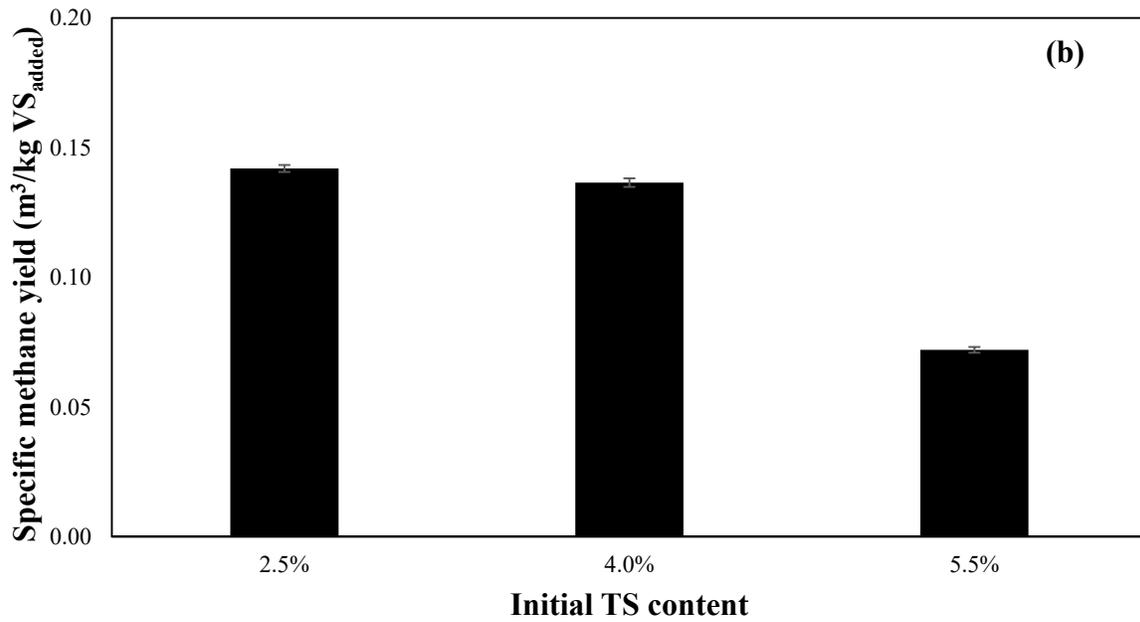
**Figure 3.** Influence of TS content on specific gas yield of anaerobic co-digestion of swine manure and corn stover. (a) Specific biogas yield; (b) Specific methane yield.
