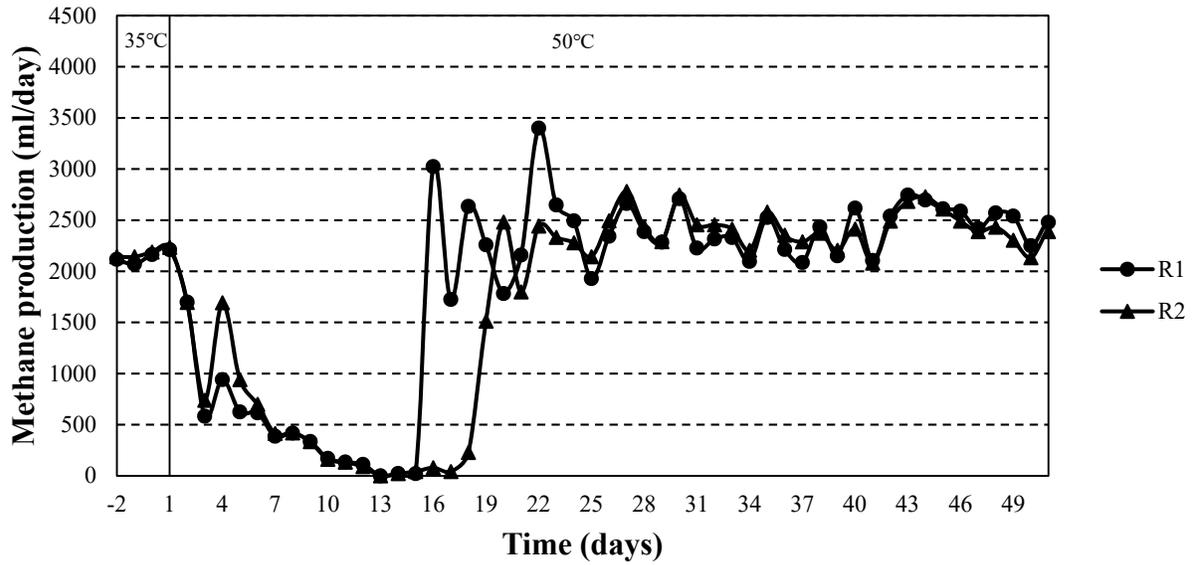
**Figure 1.** Daily methane production in anaerobic reactors treating swine wastewater and corn stover during the transition from mesophilic (35 °C) to thermophilic conditions (50 °C).
