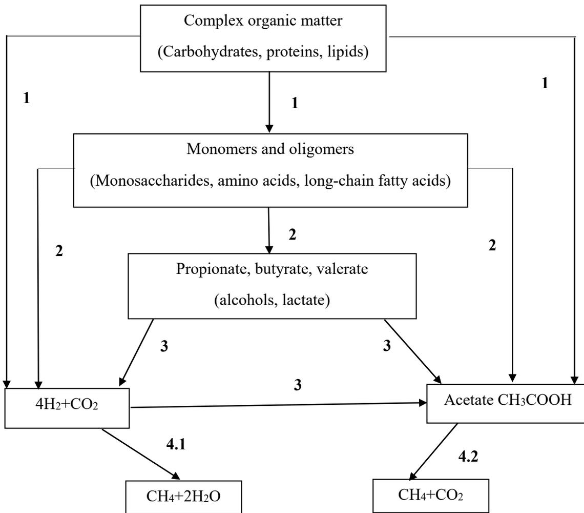
**Figure 1.** Anaerobic digestion of organic materials into biogas: 1. Hydrolysis; 2. Acidogenesis; 3. Acetogenesis; 4. Methanogenesis; 4.1 Hydrogenotrophic methanogenesis; 4.2 Aceticlastic methanogenesis.
