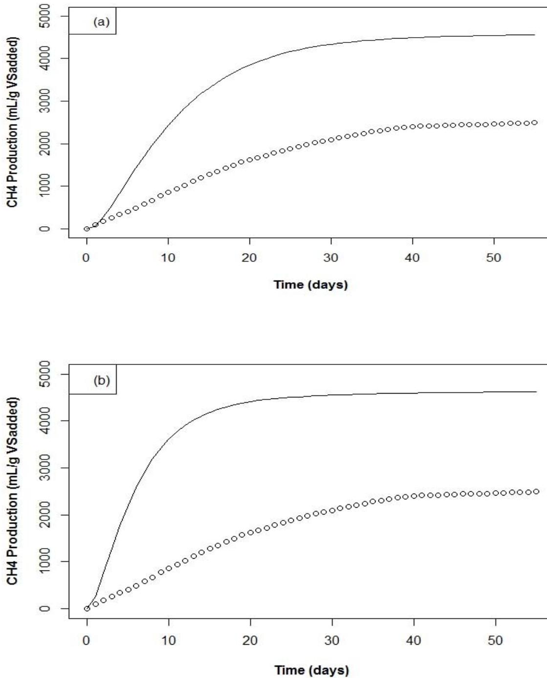
**Figure 3.** Simulation of methane generation in batch experiments using different values of parameters: (a) mesophilic kinetic values; (b) calculated thermophilic kinetic values (○ experimental data; — model simulation).
