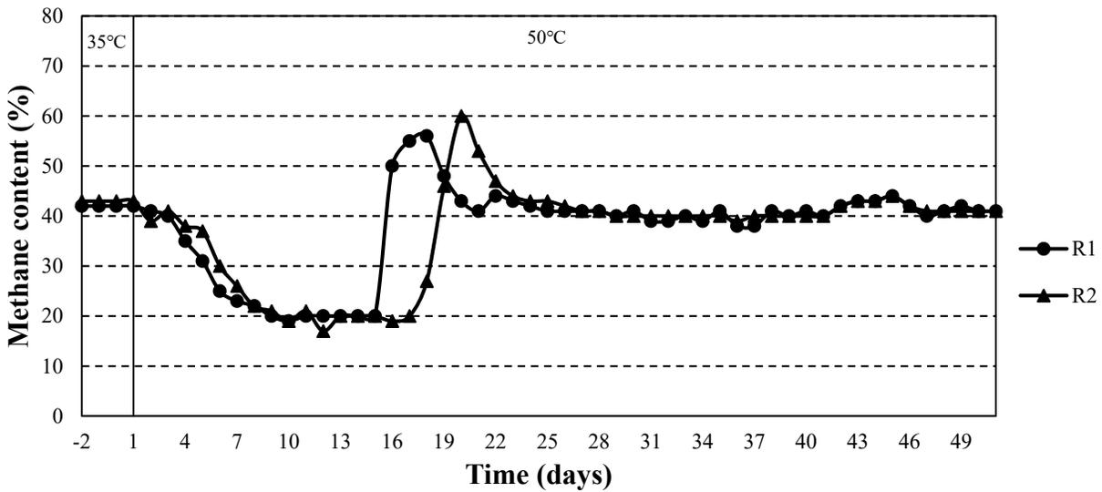
**Figure 2.** Methane content in the biogas from anaerobic reactors treating swine wastewater and corn stover during the transition from mesophilic (35 °C) to thermophilic conditions (50 °C).
