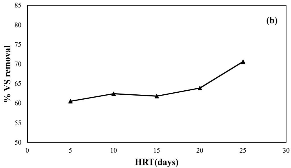
**Figure 4.** a) COD removal and b) VS reduction at different hydraulic retention times (HRTs) in a thermophilic anaerobic reactor treating swine wastewater and corn stover.
