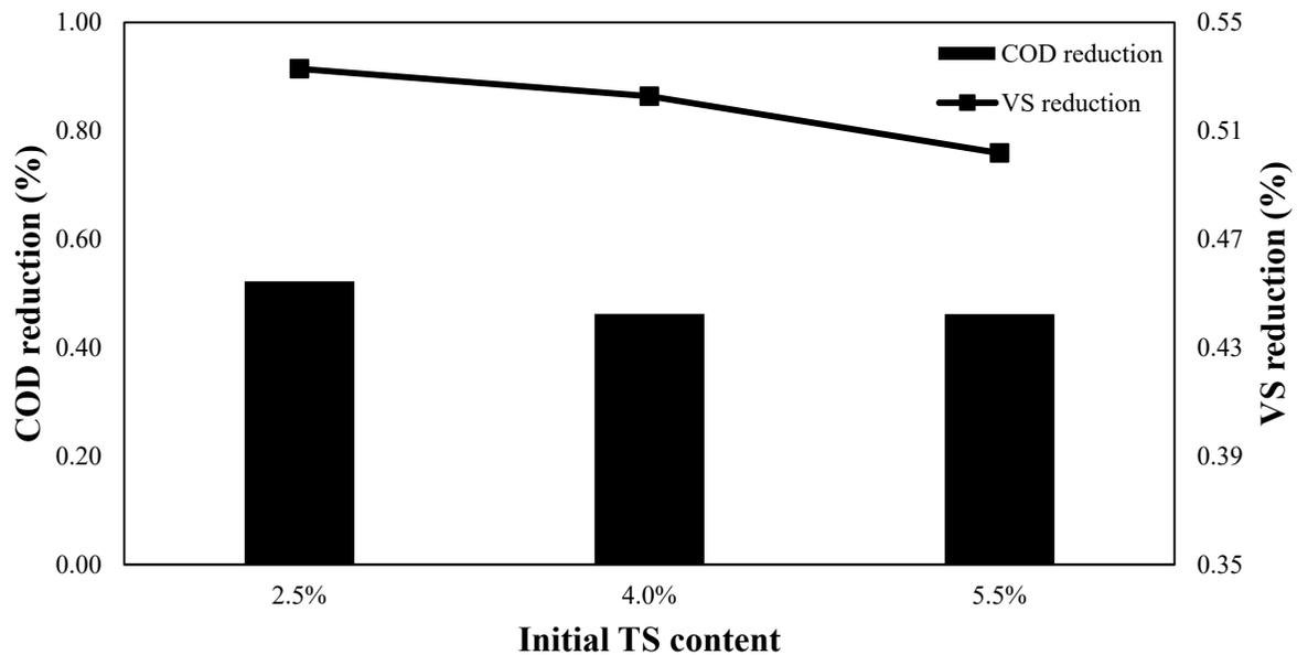
**Figure 4.** COD and VS reduction in anaerobic reactors treating swine manure and corn stover at various solid contents
