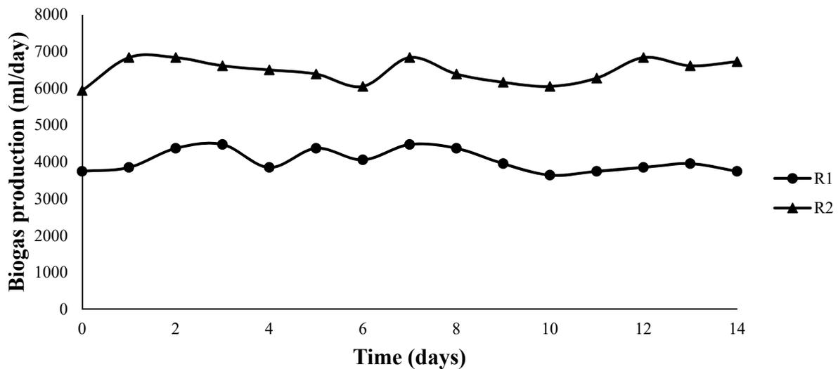
**Figure 3.** Daily biogas production in anaerobic reactors treating swine wastewater with untreated and combined NaOH and lime-treated corn stover
