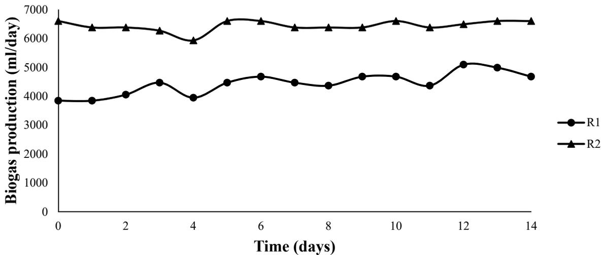
**Figure 1.** Daily biogas production in anaerobic reactors treating swine wastewater with untreated and NaOH-treated corn stover
