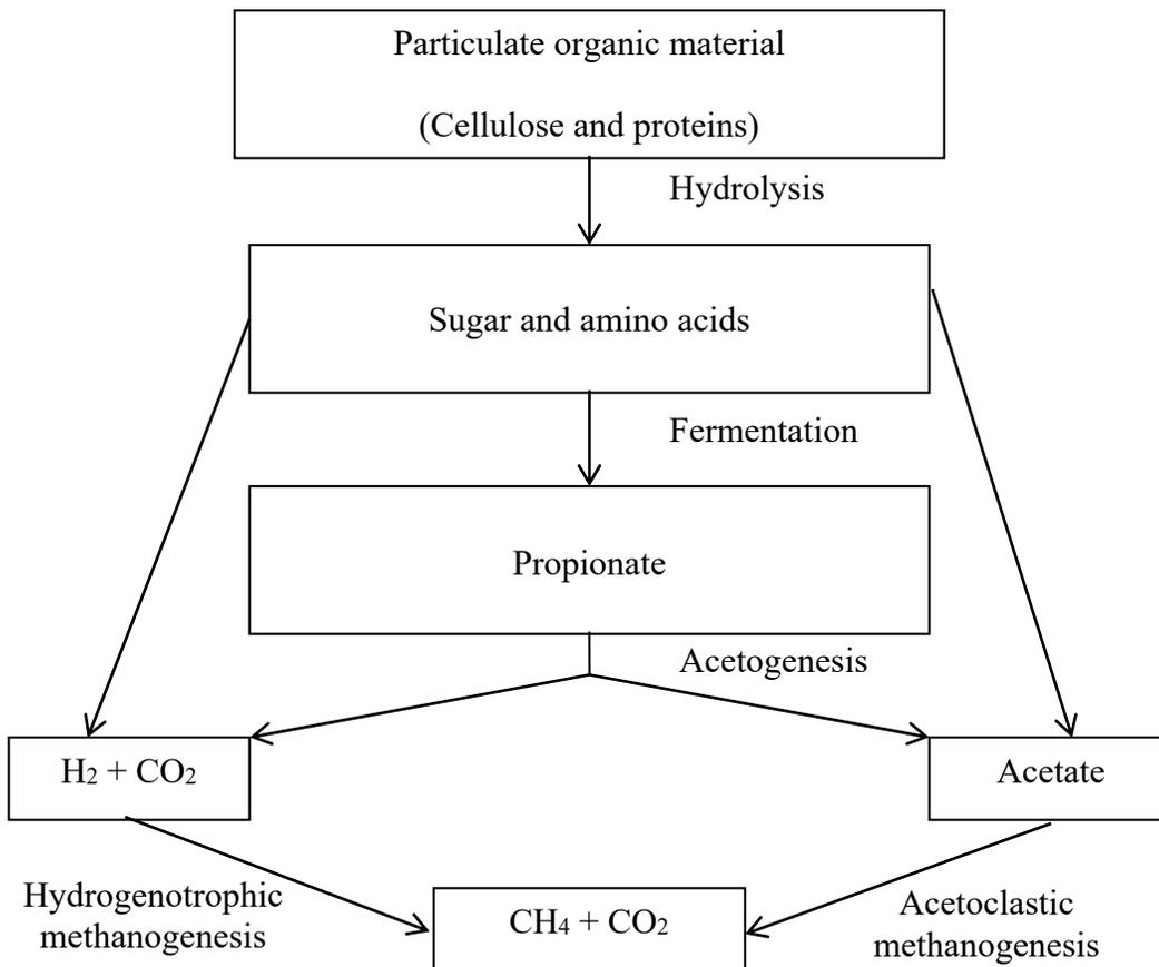
**Figure 1.** Proposed reaction scheme for the anaerobic co-digestion of swine manure and corn stover
