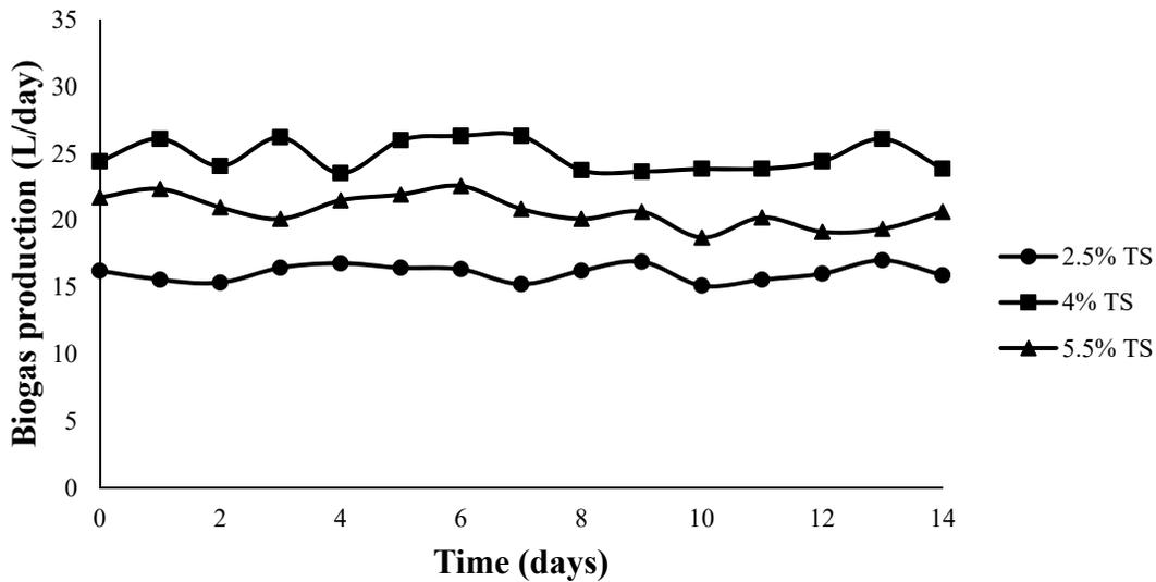
**Figure 1.** Daily biogas production in anaerobic reactors treating swine manure and corn stover at different solid contents
