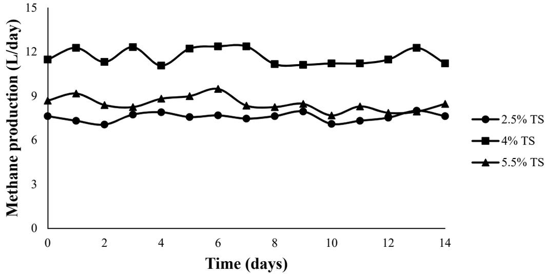
**Figure 2.** Daily methane production in anaerobic reactors treating swine manure and corn stover at different solid contents
