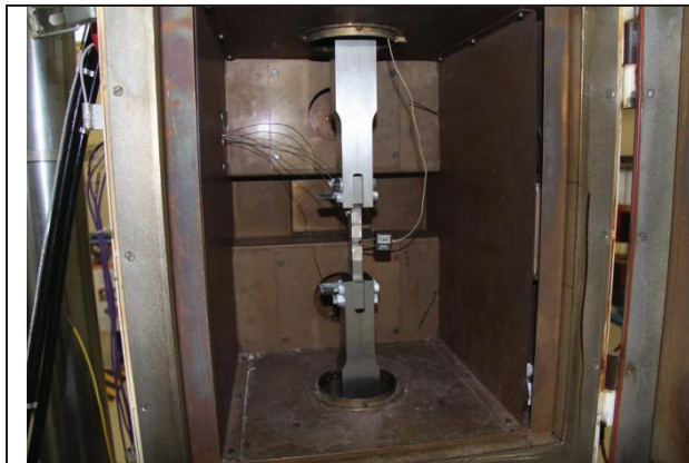
Figure 8. View of the SENT specimen in the cold chamber for low temperature tests.
