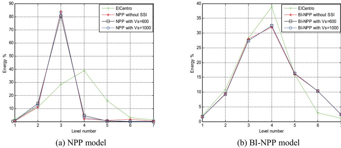
Figure 5. Energy distribution at each decomposition level of acceleration responses of nuclear power plant models.
