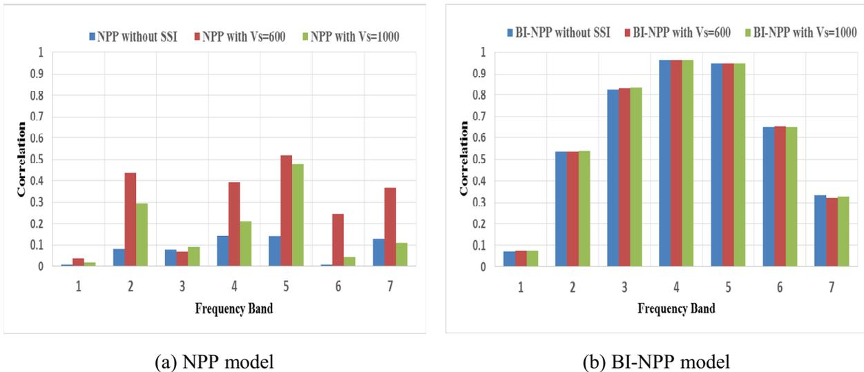
Figure 6. Degree of correlation between ground motion and acceleration response of nuclear power plant models.
