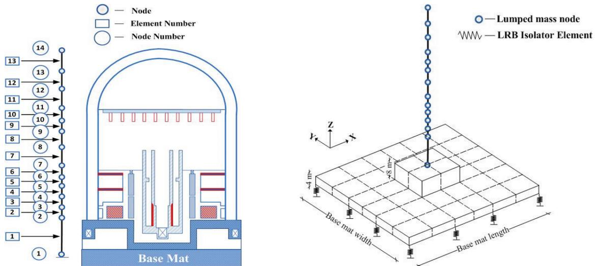
Figure 1. NPP containment building sectional elevation and stick model (left), Nuclear island base mat dimensions (right).
