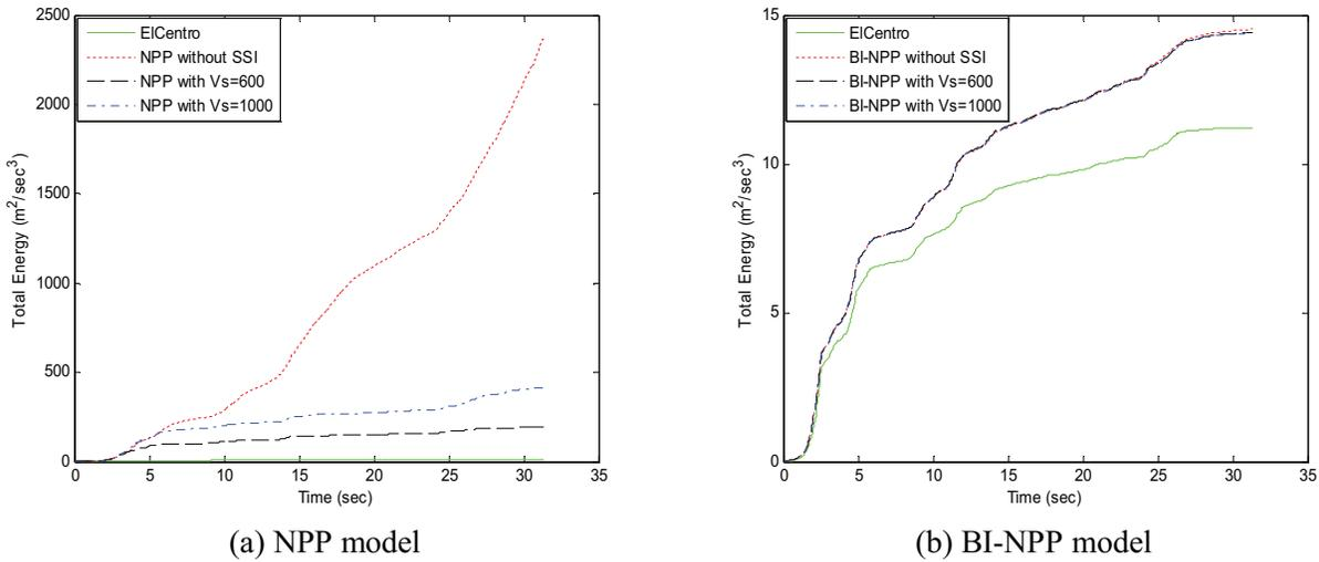
Figure 4. Total energy of acceleration responses of nuclear power plant models.
