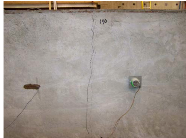
Figure 4. Cracking of OOPV+T-2.0 under axial loading
