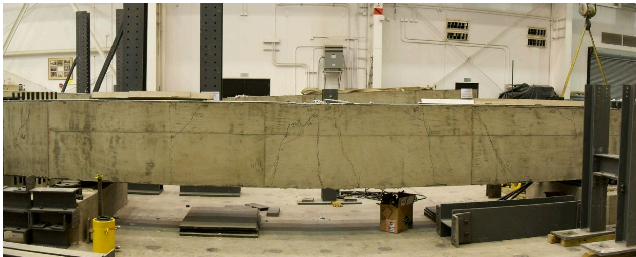
Figure 14. Cracking map of OOPV+T-3.5 after the test
