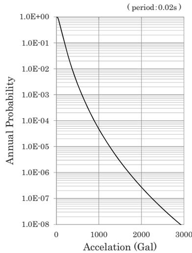
Figure 4. Seismic hazard curve
