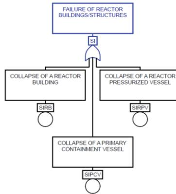
Figure 3. Example of the fault tree (BWR plant)
