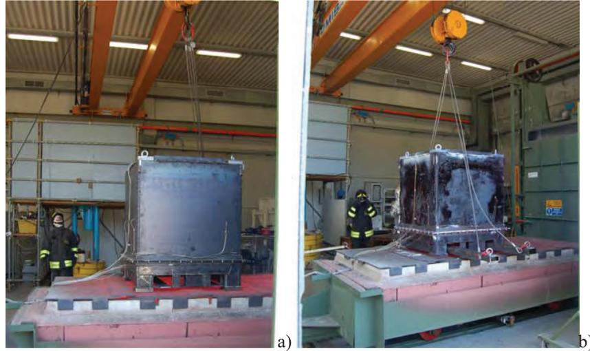
Figure 5. Positioning of the mock-up on the slide of the oven before (a) and after fire test (b) .
