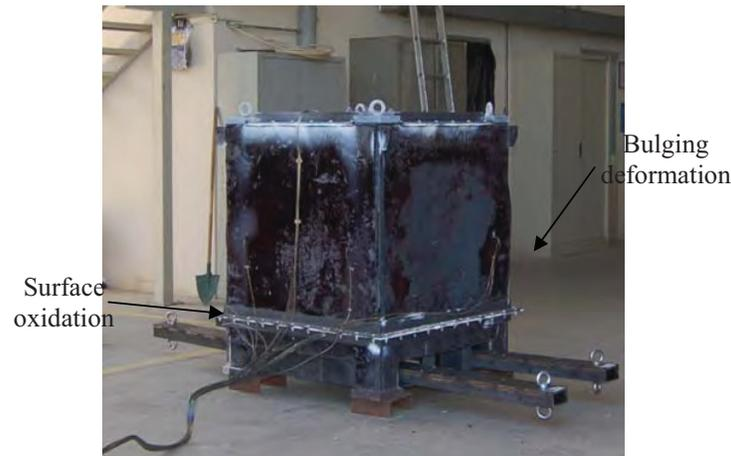
Figure 10. Overview of the mock-up after the fire test.
